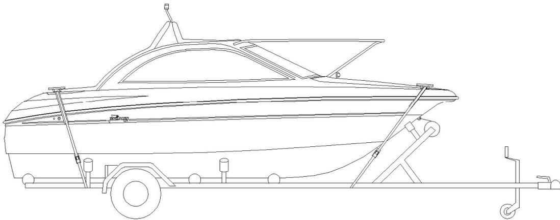
Fastening the boat onto the trailer
