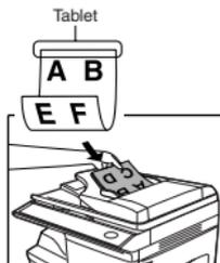
If you are faxing a two-sided tablet type original, select "ON (NON-ROTATE)".
