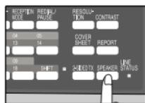
To adjust the volume, press the left and [◀] key (◻) or [▶] key (◻).
