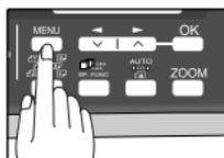
**2** Press the [◀] key (◀) or [▶] key (▶) until "5:ANTI JUNK FAX" appears, and then press the [OK] key.
