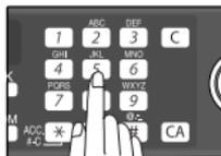
Enter the transferring fax number (maximum 40 digits) by pressing the numeric keys.
