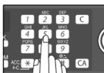
Enter the Quiet Detect Time in seconds, from 00 to 10. (setting "00" turns off Quiet Detect Time)
