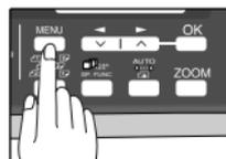
**2 Press the [←] key (L) or [→] key (R) until "2:ENTRY MODE" appears, and then press the [OK] key.**
