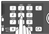
If it is not correct, press the [CLEAR] key (C) to backspace and clear one digit at a time, and then enter the correct number.
