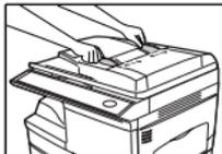
**3** Place the original(s) face up and push it gently into the document feeder tray. The top edge of the original(s) should enter the fax first.
