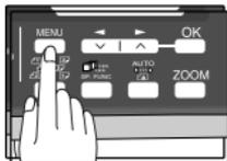
**2** Press the [◀] key (◀) or [▶] key (▶) until "0:RX DATA TRANSFER" appears, and then press the [OK] key.
