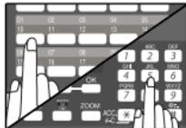
If it is not correct, press the [CLEAR] key (C) to backspace and clear two digits at a time, and then enter the correct number.
