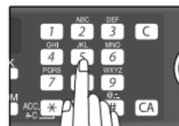
Enter the fax number (maximum of 40 digits including pauses) using the numeric keys.
