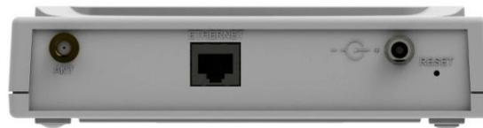
1. Connect an suitable antenna to the SMA connector. For antenna information, see [Antenna System for Cellular Devices](#).
