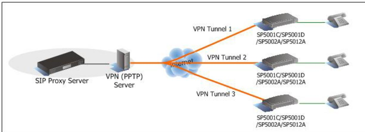
The IP telephony gateway series supports PPTP client for VPN function. It can establish VPN tunnel with PPTP server, and get access to the peer private network as if it is located in the same LAN.
