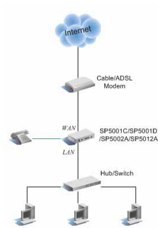
By default, the gateway is in NAT mode (router mode) and can share Internet access with PCs. Go to [ [Network / WAN Settings](#) ], and configure WAN setting according to actual condition. In default IP type of DHCP client, it requests necessary IP information from your ISP automatically.
