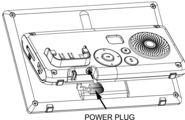
1. Insert the small plug of the power adapter into the DC socket at the bottom of the stand of the digital photo frame.
