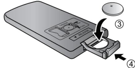
4. Slide the battery holder back into the remote control.
