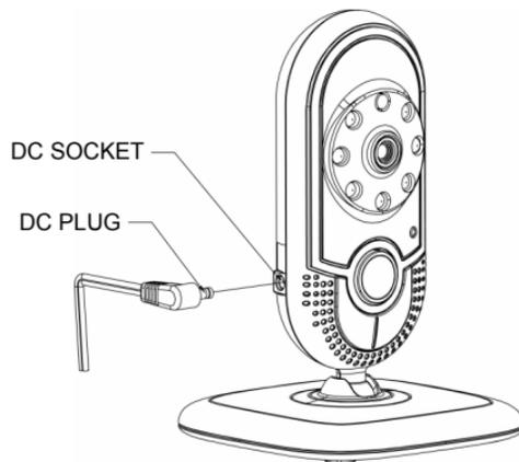
1. Insert the small plug of the power adapter into the side of the camera unit.
