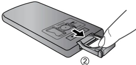
3. Insert the new battery into the battery holder. The battery must be placed with the positive pole facing upwards in the illustrated position.
