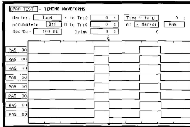
If this is the first time you have acquired data and you have not previously set up the **TIMING WAVEFORMS** menu, you will see eight labels named **RAS**. Don't worry, this is normal. To turn on the **CAS** label and delete the other six **RAS** labels, follow these steps:
