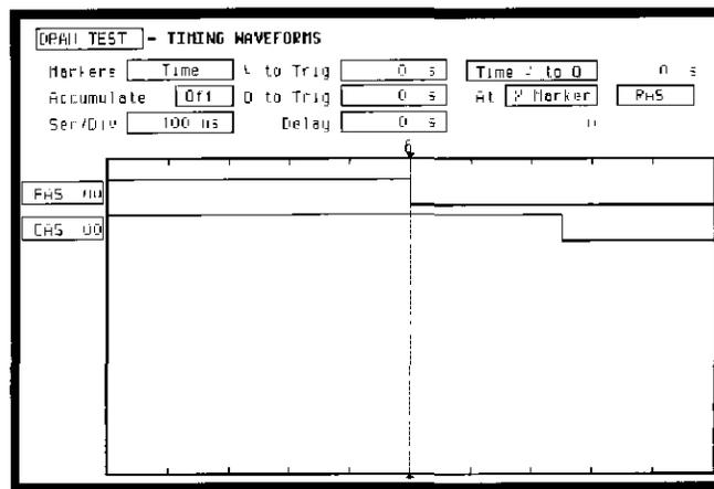
The RAS label shows you the RAS signal and the CAS label shows you the CAS signal. Notice the RAS signal goes low at or near the center of the waveform display area (horizontal center).
