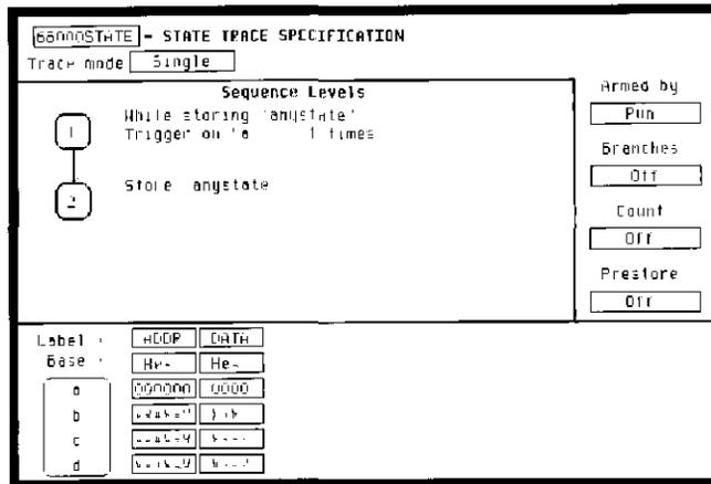
When the state analyzer is connected to your circuit and is acquiring data, it continuously stores until it sees 0000 on the address bus, then it will store anystate until the analyzer memory is filled.
