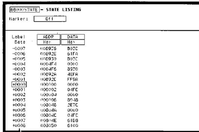
The screenshot shows a window titled "68000STATE - STATE LISTING" with a "Markers" control set to "Off". Below this is a table with three columns: "Label", "ADDR", and "DATA". The "Label" column contains state line numbers from -0007 to +0008, with +0000 highlighted. The "ADDR" column shows hexadecimal addresses, and the "DATA" column shows hexadecimal data values.
