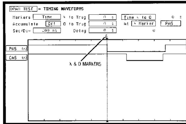
**The ▼** The ▼ (inverted triangle) indicates the trace point. Remember, trace point = trigger + delay. Since delay in this example is 0.000 s, you will see the negative-going edge of the RAS signal at center screen under the ▼.
