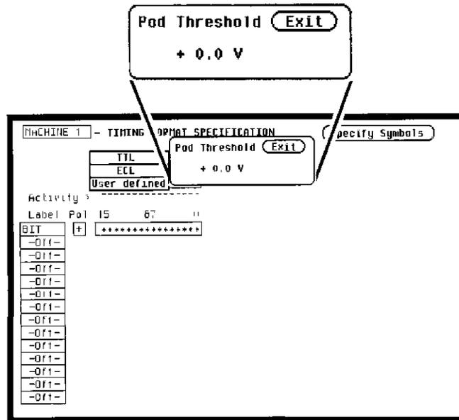
You can enter your desired threshold with either of two methods when the pod threshold pop-up is open. The first method is to rotate the **KNOB** until your desired threshold is displayed. Rotating the **KNOB** increments or decrements the value in small increments.
