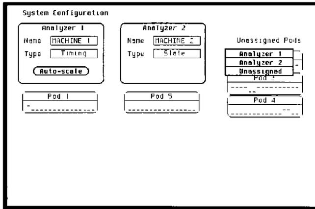
3. Place the cursor on Analyzer 2 and press **SELECT**. The pop-up closes and your desired pod is now assigned to analyzer 2.
