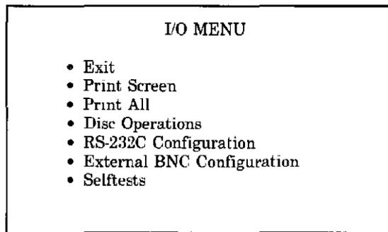
**Print Screen** The **Print Screen** option prints only what is displayed on screen at the time you initiate the printout. In the Print Screen mode, the printer uses its graphics capabilities so the printout will look just like the logic analyzer screen with only one exception: the cursor will not print.
