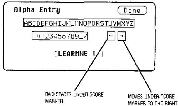
To move the under-score marker to the right, you either place the cursor on a desired character and press **SELECT**, or place it on the right arrow and press **SELECT**.
