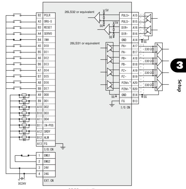
■ I/O wiring diagram
