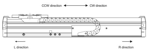
• On the PHASER series, the CW direction is to the right when viewed from the cable carrier side.
