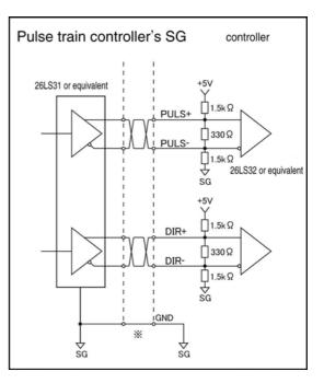
\* The robot controller's SG must be connected to the pulse train controller's SG. The SG terminals (pin No. A14 and B14) are isolated from 24G (pin No. 4 of EXT. CN). Wire each of them securely.
