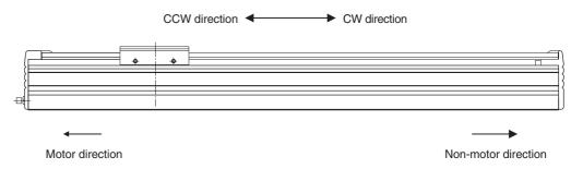
• On the FLIP-X series, CW is the clockwise direction as seen from the load, and CCW is the counterclockwise direction.
