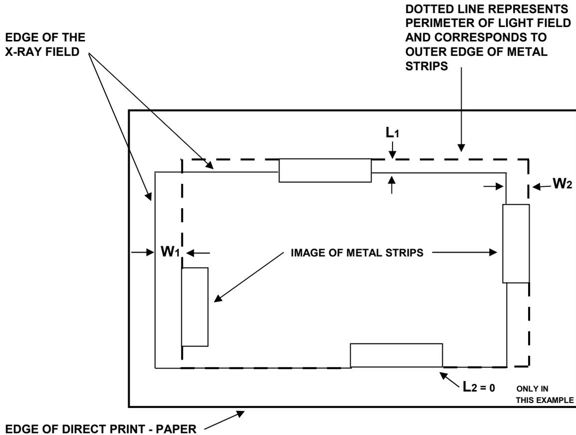
FIGURE 5.3 LIGHT FIELD vs. X-RAY FIELD ERROR MEASUREMENTS
