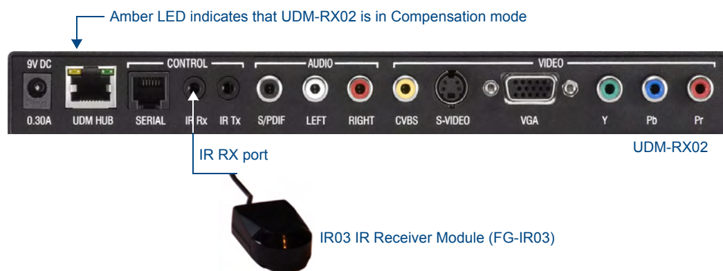
FIG. 26 UDM-RX02 with IR03 IR Receiver Module
