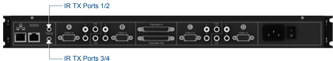
FIG. 53 IR TX ports for locally connected devices
