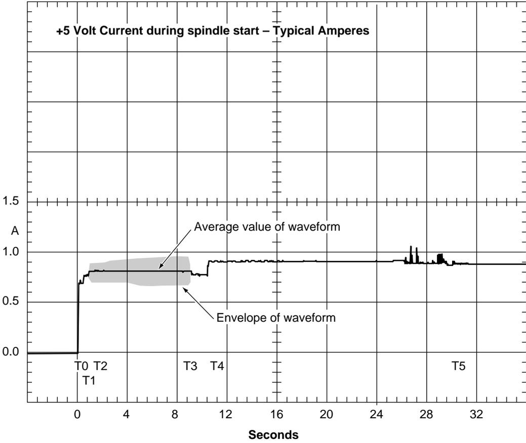
Figure 4. Typical Cheetah 73FC drive +5V current profile
