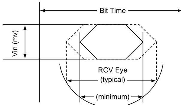
Figure 18. Receive eye diagram
