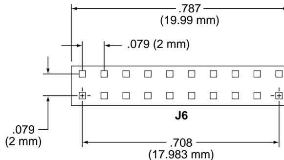
Figure 15. J6 connector dimensions
