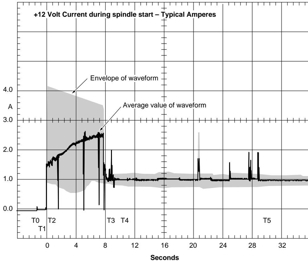
**Figure 3. Typical Cheetah 73FC drive +12V current profile**
