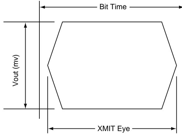
Figure 17. Transmit eye diagram
