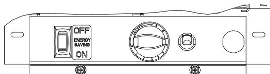
observed on the door opening, press the energy saver switch to the OFF position, to increase the amount of heat (red portion of the rocker switch will be visible).
