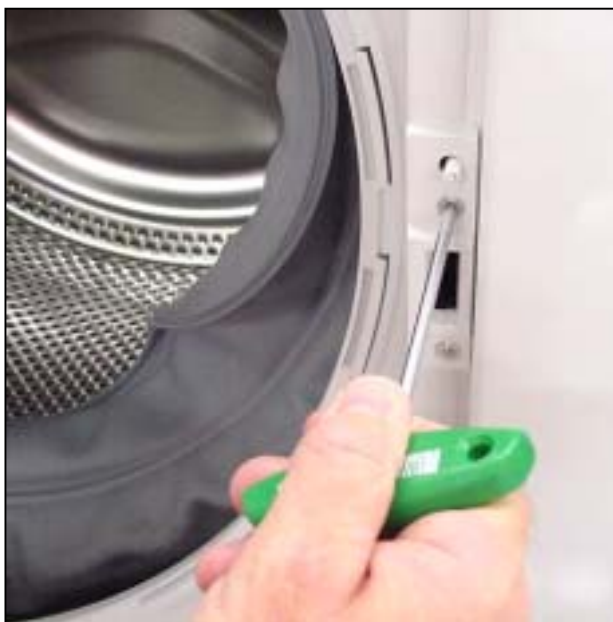
Remove door latch screws
