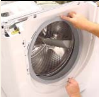
Remove front seal spring
