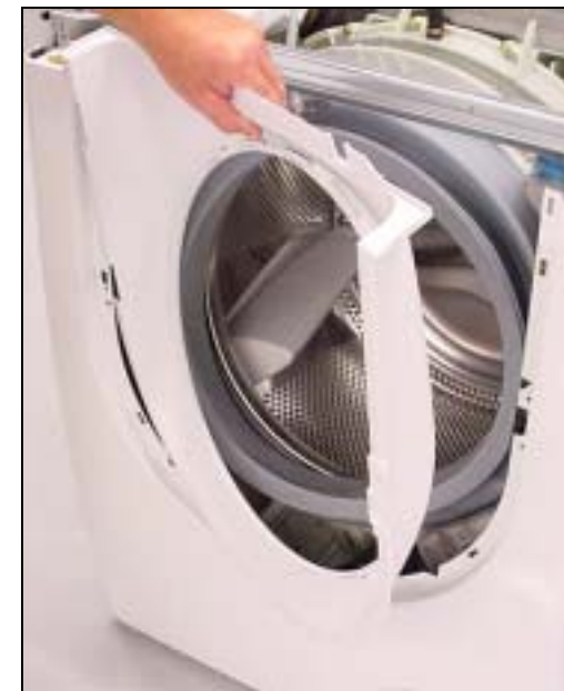
Removing front shield
