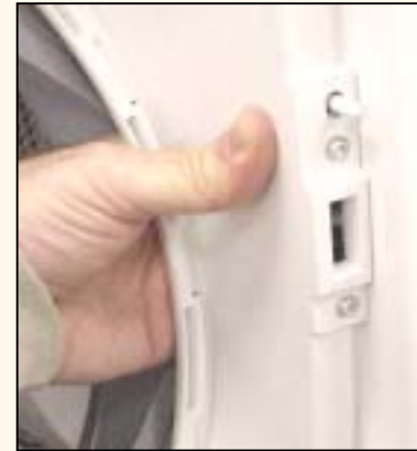
Push onto back of door lock until it clicks open
