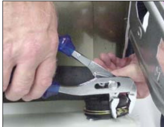
Disconnect main water inlet hose
