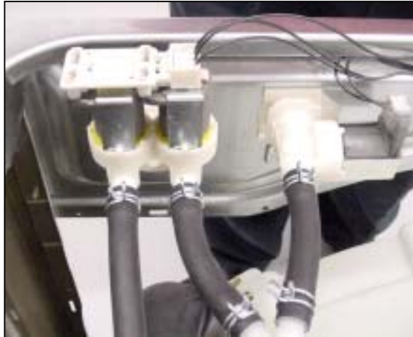
Disconnect water inlet valve hoses
