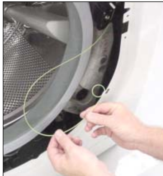
Door latch manual release
