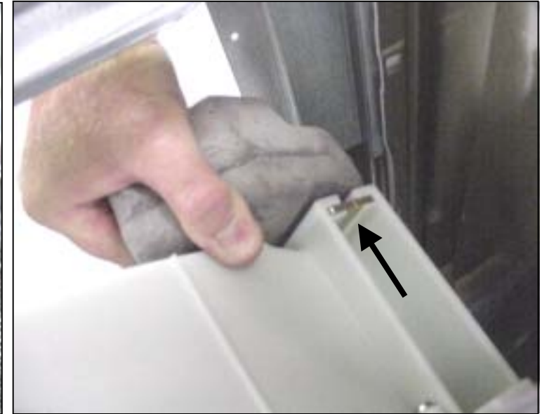
Note counterweight screw bushings in tub
