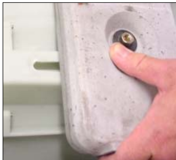
Slide out counterweight
