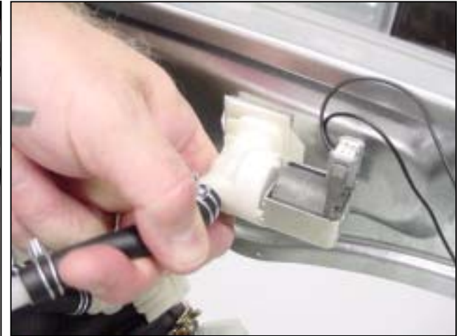
Disconnecting hot water valve hose
