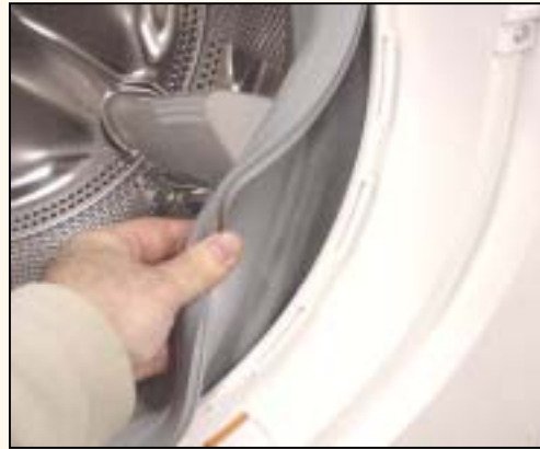
Move door seal for access
