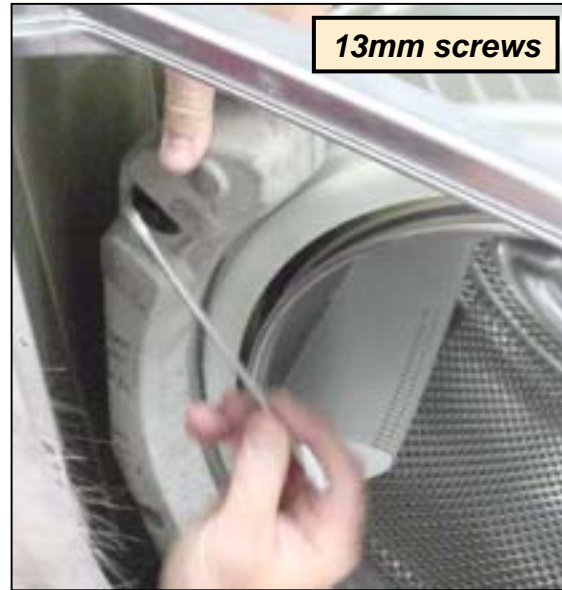
Removing counterweight screws
