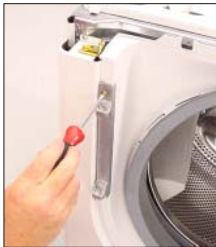
Remove hinge screws
