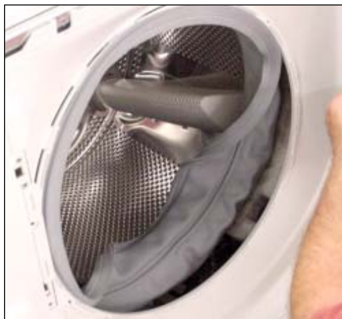
Carefully remove front shield
