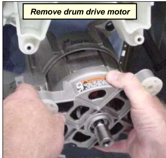
Showing drum drive motor mounts
