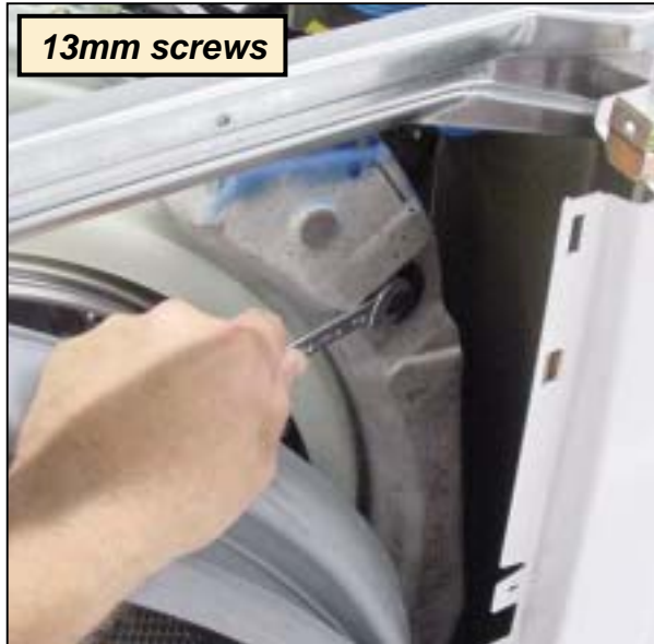
Remove front counterweight screws
