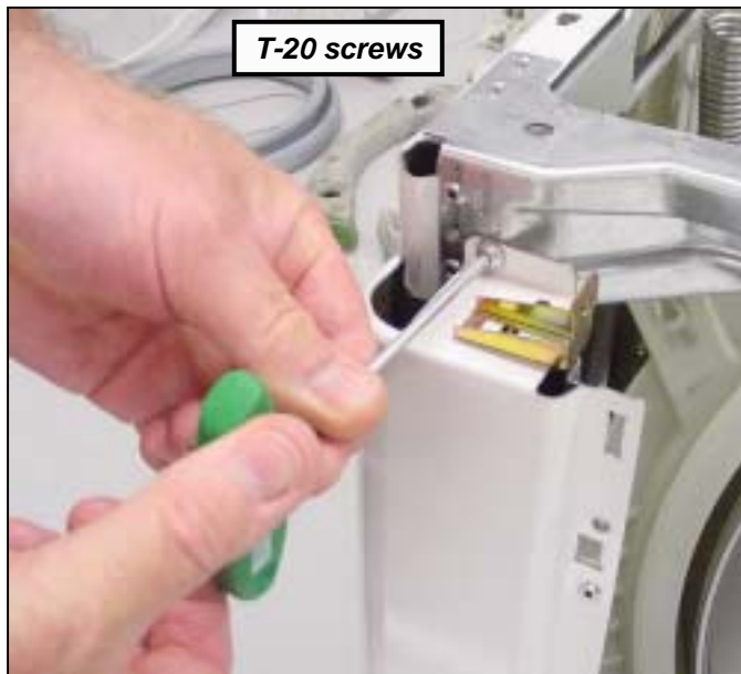
Remove top front panel screws
