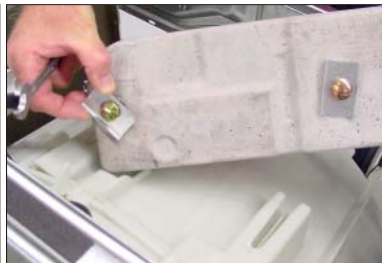
Note counterweight bushing slots in tub
