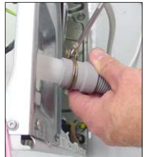
Disconnect drain hose
