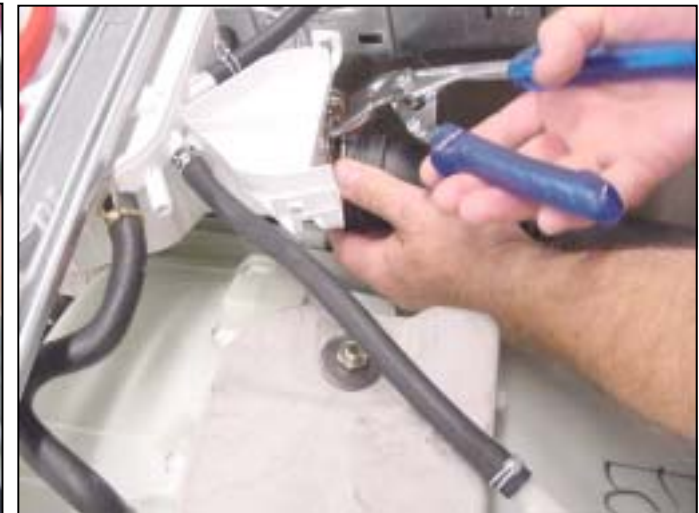
Disconnecting main water inlet hose
