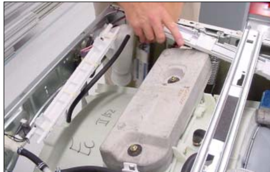
Top counterweight must be removed
