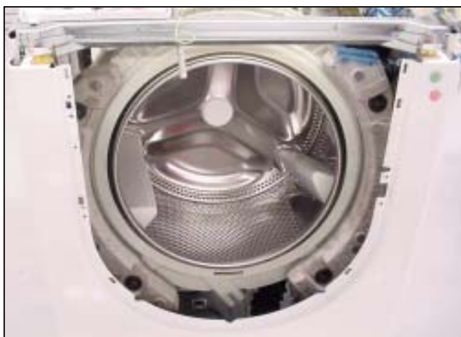
Remove front panel
