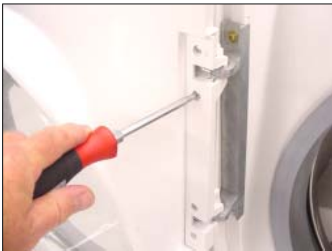
Remove hinge cover screws
