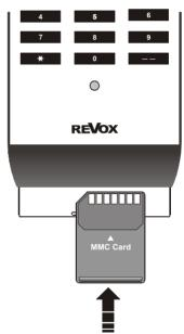
Press the card gently into the compartment to release it, if you want to remove it. The compartment has an eject mechanism that then pushes the card out.
