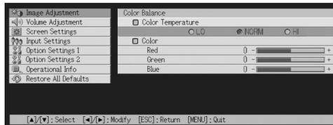
3. Use the [◀] and [▶] keys to adjust the color temperature.
