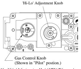
Figure 11. 'Hi-Lo' Adjustment on Model ME34-BV gas valve.
