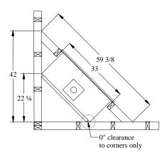
Figure 3. Corner framing dimensions.
