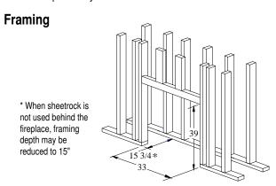
Figure 2. Framing dimensions.
