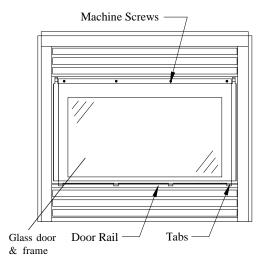
**Figure 10b.** Removing or installing the glass door.
