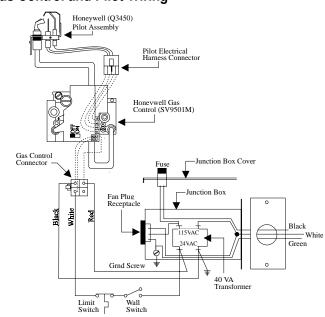
**Figure 6.** Wiring for the ME34-BV-I with Honeywell gas control and pilot.
