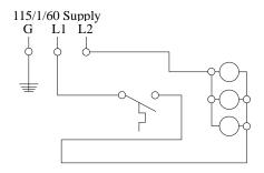
Figure 7b. Wiring schematic for optional fan kit.
