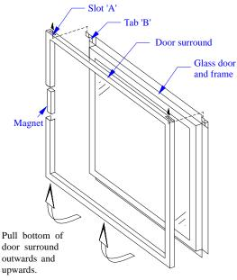
Figure 10a. Removing or installing the door surround.
