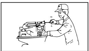
Non-reusable items Always use new gaskets, packings, Orings, split-pins, circlips, etc., on reassembly.
