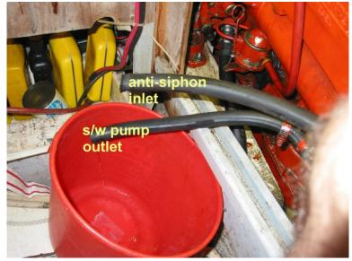
2. Disconnect the anti-siphon inlet (the raw water connection into the exhaust elbow at the elbow); this means you're back flushing through the oil cooler because the oil cooler inlet hose is about 2 inches and would be tough to remove.
