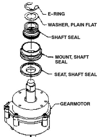
FIGURE 9. SHAFT SEAL
