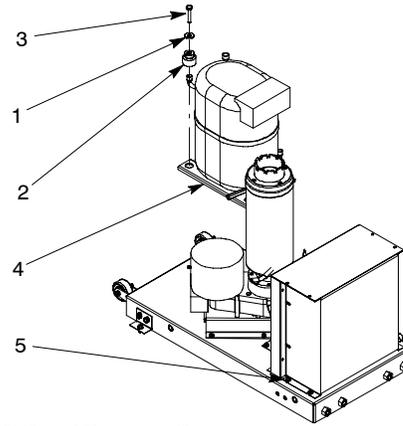
**FIGURE 18. COMPRESSOR COMPONENTS**
