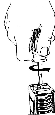
**FIGURE 6. ADJUSTMENT SCREW**
