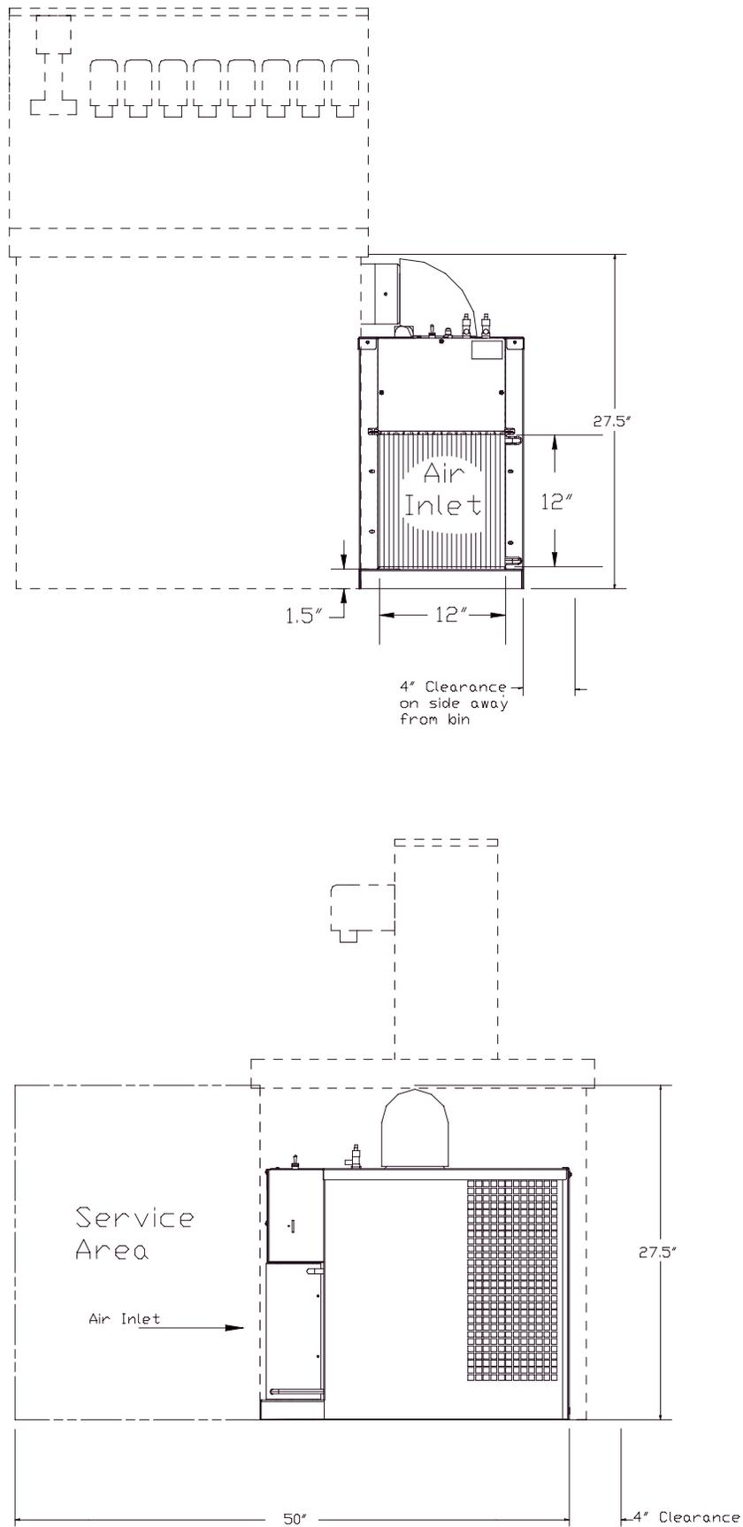
**FIGURE 1. CLEARANCE REQUIREMENTS**
