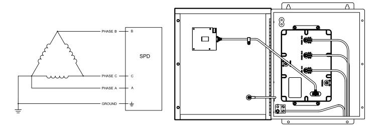
Figure 7: Three-Phase, 3-Wire, High-Resistance Grounded Delta Installation
