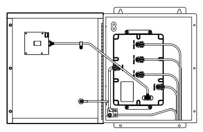
Figure 5: Three-Phase, 3-Wire, Delta Installation
