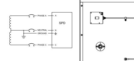
Figure 9: Three-Phase, 3- or 4-Wire, Grounded Wye Installation with Integral Disconnect
