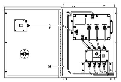
Figure 11: Three-Phase, 3-Wire, Delta Installation with Integral Disconnect
