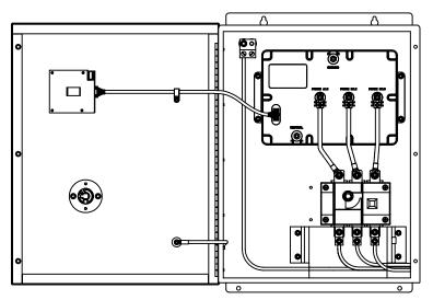
Figure 13: Three-Phase, 3-Wire, High-Resistance Grounded Delta Installation with Integral Disconnect
