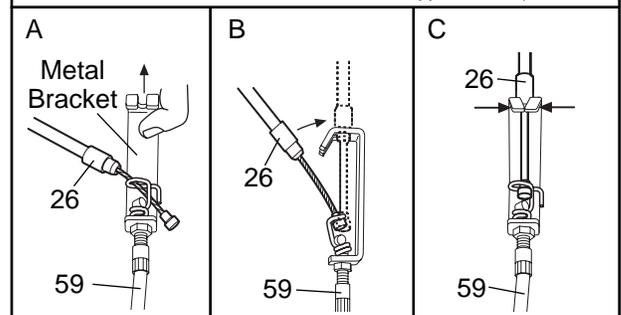
3. Insert the pulse wires beneath the indicated bracket on the Upright (3) and up out of the hole in the top of the Upright. Attach the T-Handle (10) to the Upright with two M6 x 16mm Screws (54) and two M6 Black Nylon Locknuts (55).
