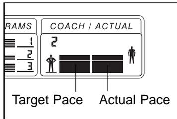
The three graphs on the console show how the target pace will change during the programs. During the Aerobic program (program 2), for example, the target pace will gradually increase during the first half of the program, and gradually decrease during the last half of the program. Each program will last for twenty minutes.
