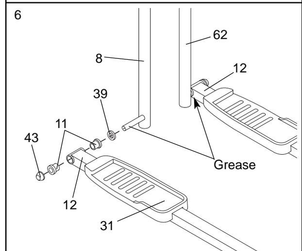
Slide a Handlebar Spacer (39) and the Pedal Arm (12) with the Left Pedal (31) onto the Left Handlebar (8) as shown. Make sure that there are two Pedal Arm Bushings (11) in the Pedal Arm. (Note: These parts fit tightly; it may be helpful to use a rubber mallet). Next, refer to the PART IDENTIFICATION CHART on page 5 and identify the 3/4" Axle Caps (43). Tap a 3/4" Axle Cap onto the Left Handlebar.
