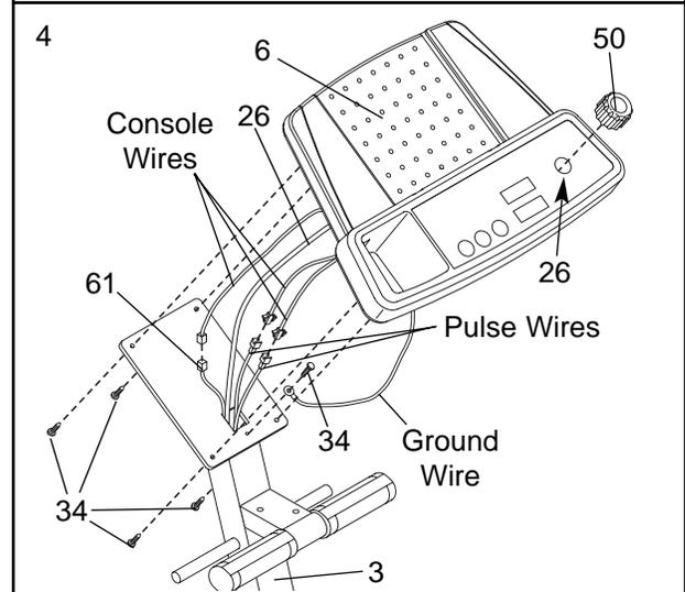
Pull any slack Resistance Cable (26) up out of the Upright (3) and push it into the Console (6). Feed the slack Extension Wire (61) down into the Upright. Attach the Console to the Upright with four M4 x 16mm Screws (34). **Be careful to avoid pinching the wires or pinching or kinking the Resistance Cable.**
