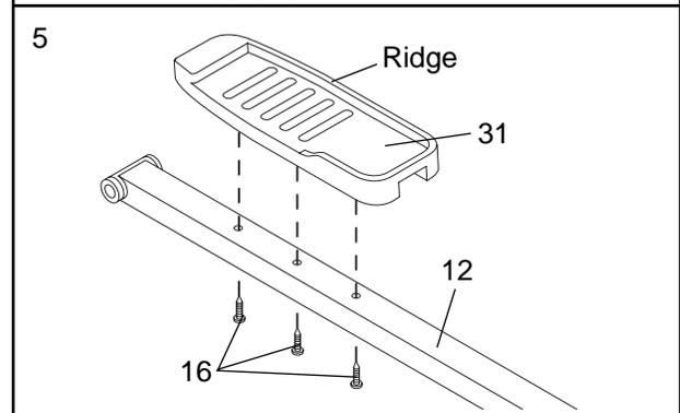
Repeat this step to attach the Right Pedal to the other Pedal Arm (not shown).
