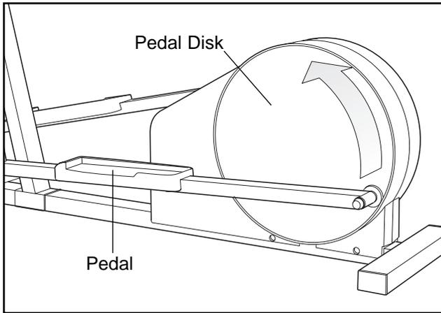
To dismount the elliptical trainer, allow the pedals to come to a complete stop. **CAUTION: The elliptical trainer does not have a free wheel; the pedals will continue to move until the flywheel stops.** When the pedals are stationary, step off the highest pedal first. Then, step off the lowest pedal.
