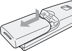
**1** Press in on the battery cover release and slide the cover down until it comes off.
