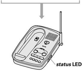
**5** Make sure that the "**status**" LED lights. If the LED doesn't light, check to see that the AC adapter is plugged in and that the handset makes good contact with the base charging contacts.
