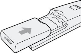
**3** Slide the battery cover forward until it snaps into place.
