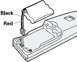
**2** Connect the battery pack connector with the correct polarity (black and red wires), then insert the battery pack into the battery compartment.
