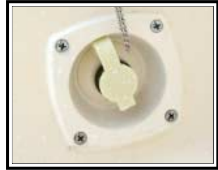
Shore Water Connection
