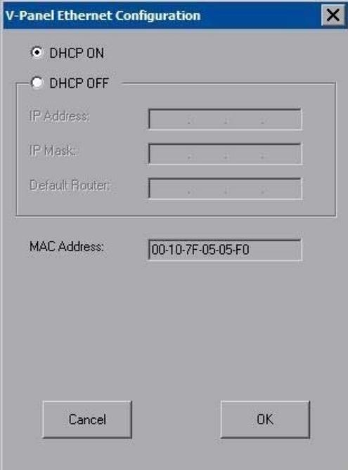
The screenshot shows a window titled "V-Panel Ethernet Configuration". At the top, there are two radio buttons: "DHCP ON" (which is selected) and "DHCP OFF". Below these, there are three input fields: "IP Address:", "IP Mask:", and "Default Router:". These fields are currently disabled (grayed out). Below these fields is a "MAC Address:" field with the value "00-10-7F-05-05-F0". At the bottom of the window, there are two buttons: "Cancel" and "OK".
