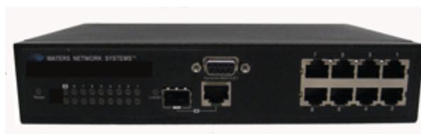
The switch provides eight switched auto-sensing 10/100Base-TX RJ45 ports plus one mini GBIC and one 10/100/1000Base-TX port. The switch provides nine usable ports. The ninth port can be used for 1000Base-SX fiber connectivity or for 10/100/1000Base-TX connectivity.
