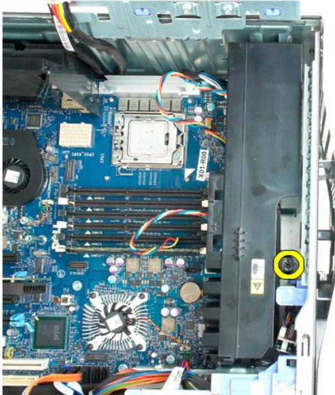
7. Remove the fan assembly from the computer
