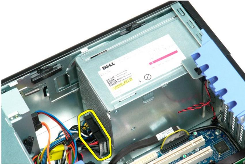
6. Push down and hold the power supply release clip (1), then slide the power supply toward the center of the computer (2).
