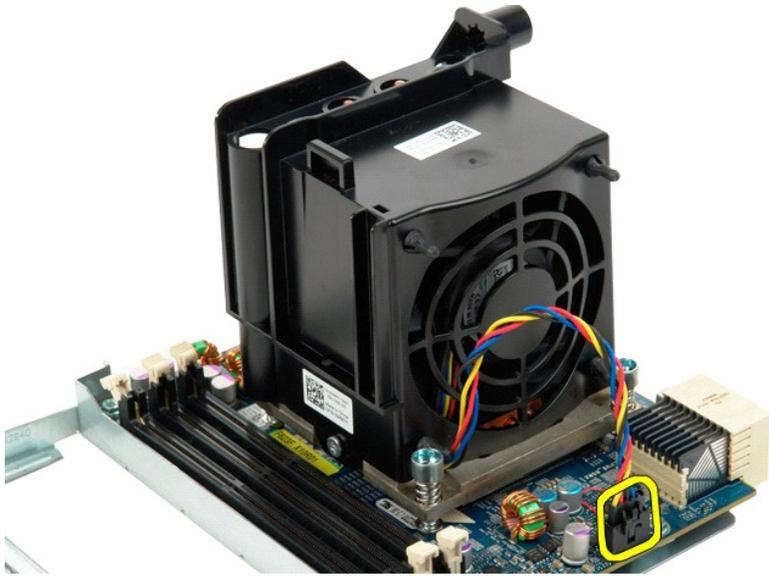
12. Loosen the four captive screws on the dual processor heat sink/fan assembly.
