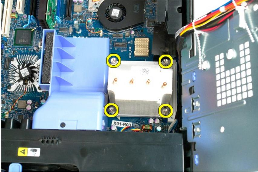
5. Lift the heat sink straight up and remove the heat sink from the computer.
