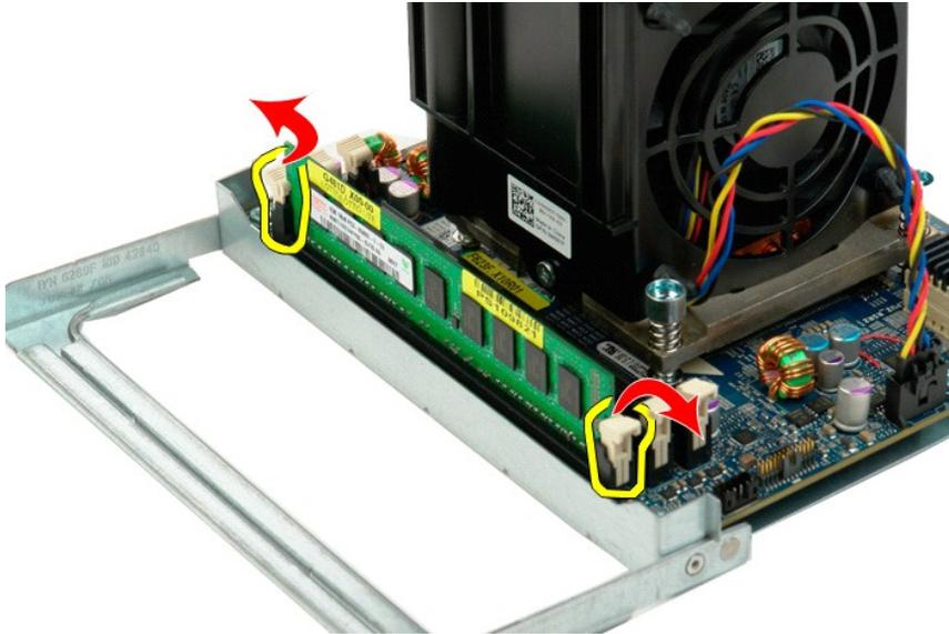
10. Remove the first memory module from the dual processor board, and repeat with any remaining memory modules.
