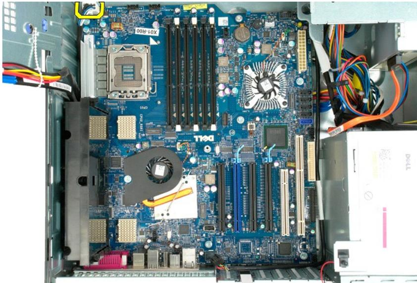
15. Remove the three screws that secure the dual processor riser to the system board.
