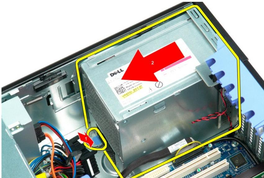
7. Remove the power supply from the system at an angle.
