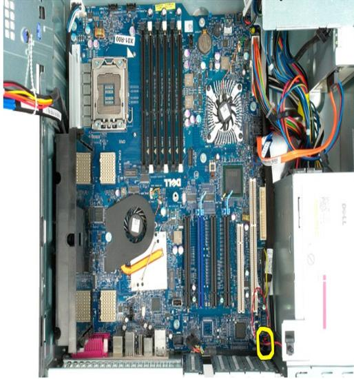
14. Disconnect the power supply data cable from the system board.
