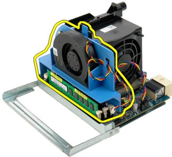
9. Gently press down on the memory module release tabs to release the first dual processor memory module from the connector.
