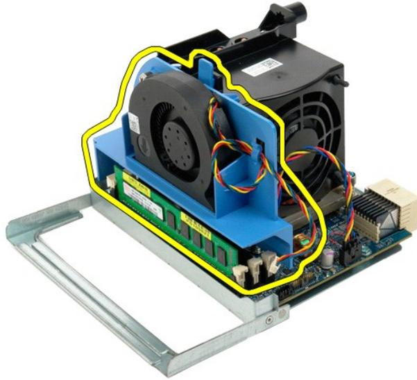
8. While pressing on the blue release tab, remove the dual processor fan assembly from the dual processor assembly.
