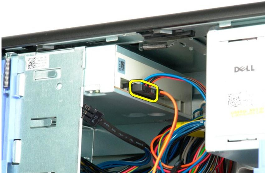
4. Disconnect the data cable from the back of the optical drive.
