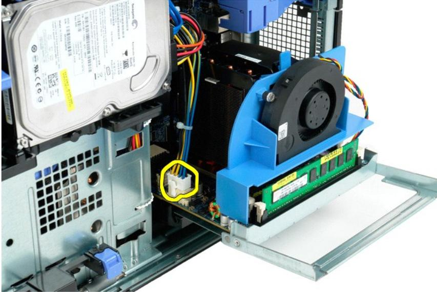
6. Remove the dual processor riser completely from the computer.
