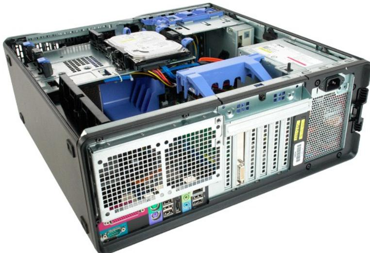
3. Remove the four screws securing the power supply on the outside of the computer.
