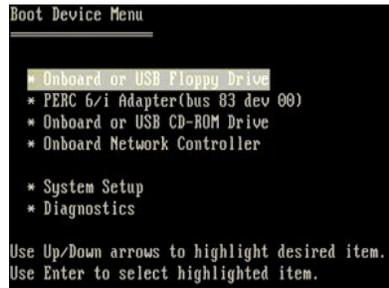
As with previous Dell Precision™ workstation platforms, your computer includes a one-time boot menu. This feature offers a quick and convenient method with which to bypass the System Setup-defined boot device order and boot directly to a specific device (e.g., floppy, CD-ROM, or hard drive).
