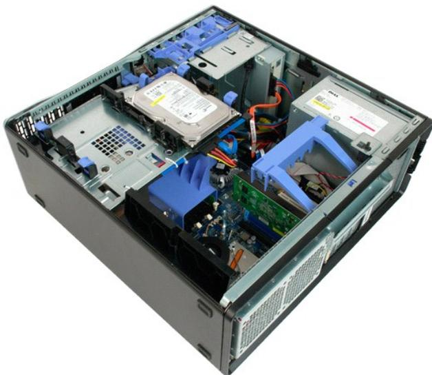
3. Disconnect the power cable from the first hard drive.
