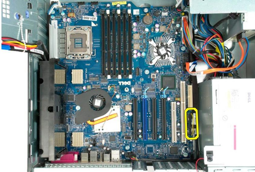
12. Disconnect the hard drive and optical drive data cables from the system board.
