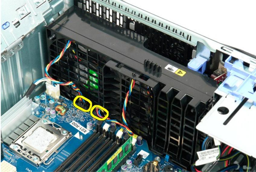
6. Remove the screw that secures the front fan assembly.
