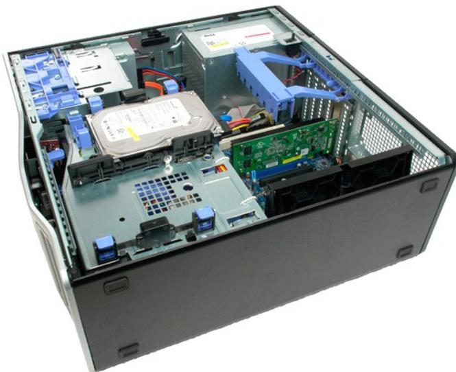
3. Squeeze the release tabs, then lift the expansion card retention arm away from the computer.
