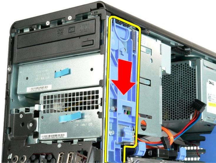
6. Slide the optical drive out of the front of the chassis, and remove from the computer.
