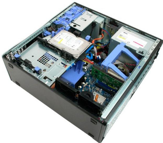
3. Pull up on the front bezel release tab.
