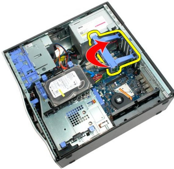
5. Disconnect the power supply cable from the power supply.
