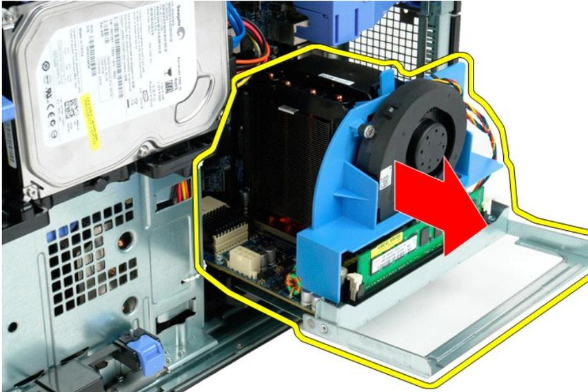
7. Disconnect the dual processor fan cable from the dual processor board.
