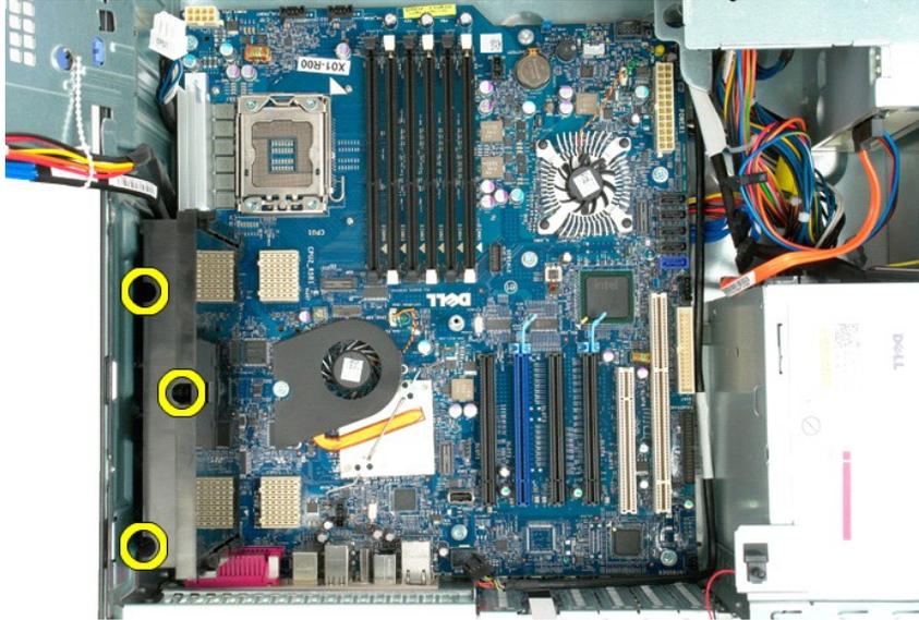
16. Remove the dual processor riser.
