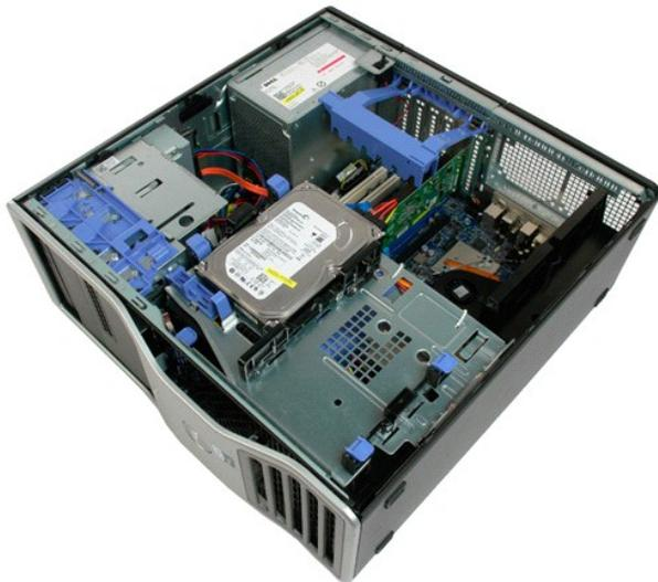
3. Press the hard drive release lever toward the bottom of the computer.
