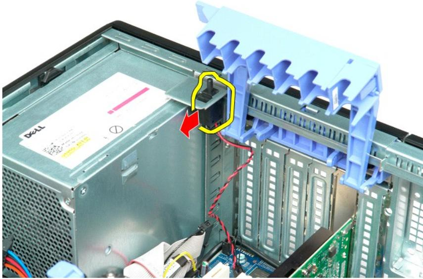
6. Remove the intrusion switch from the computer.
