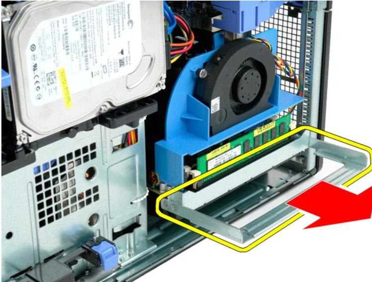
5. Disconnect the power cable from the dual processor board.
