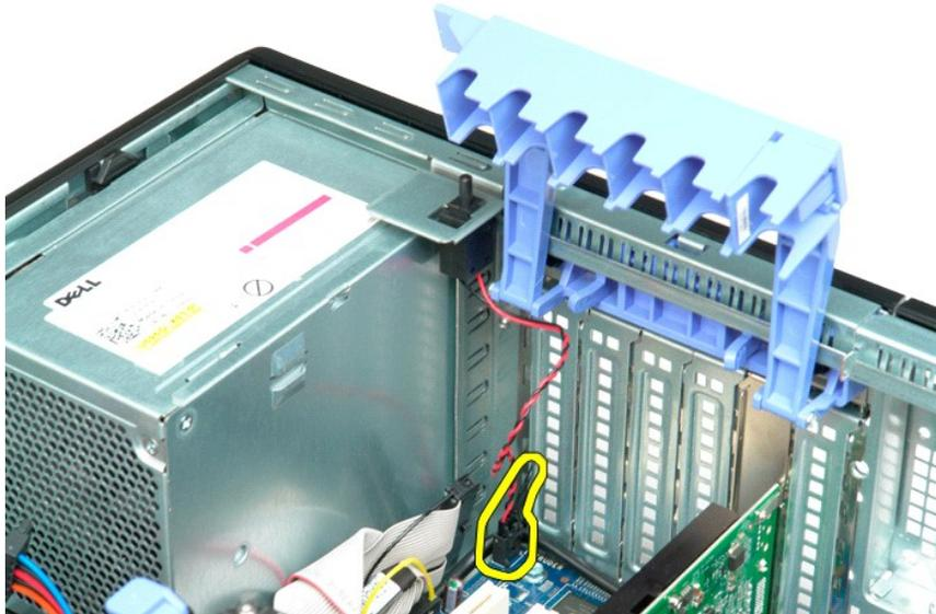
5. Slide the intrusion switch toward the center of the computer.
