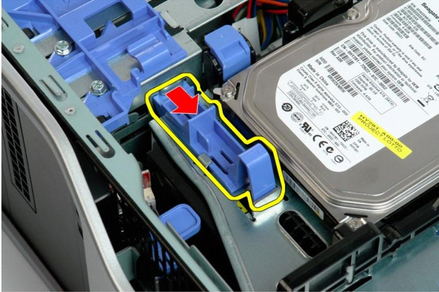
4. Lift and rotate the hard drive tray toward the bottom of the computer.
