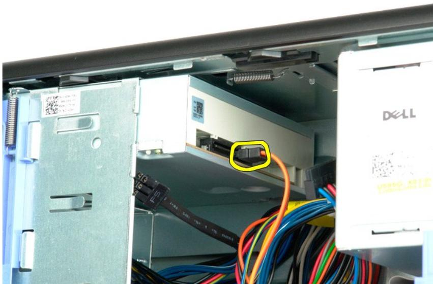
5. Press down on the sliding-plate lever and hold.
