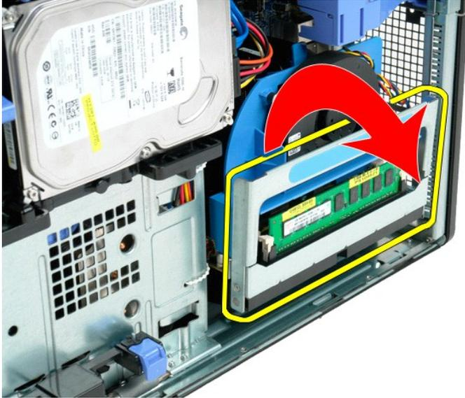
4. Carefully slide the dual processor riser halfway out.
