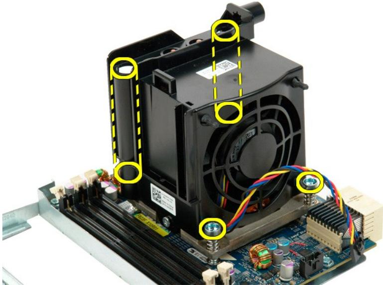
13. Remove the dual processor heat sink fan assembly from the dual processor riser board.
