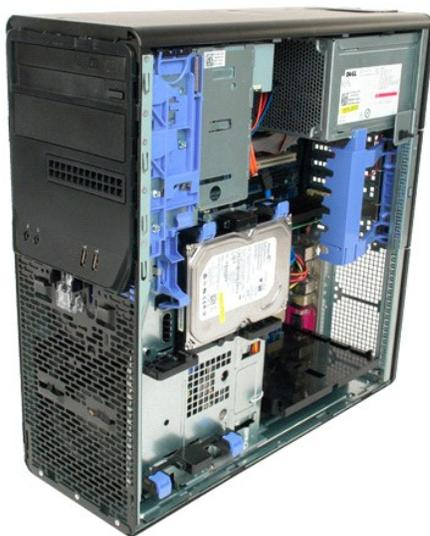
3. Press and hold the sliding-plate lever toward the base of the computer to release the drives bezel.
