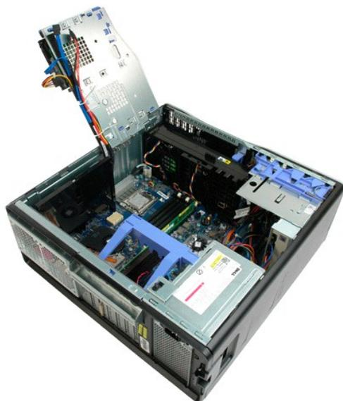
5. Disconnect the two fan cables from the system board.
