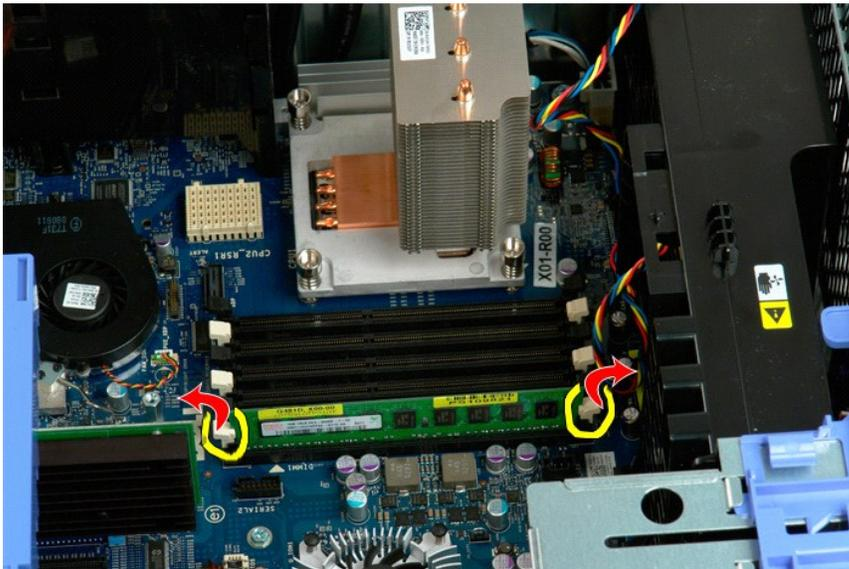
6. Lift the first memory module straight up and out of the computer, and repeat for any remaining memory modules.
