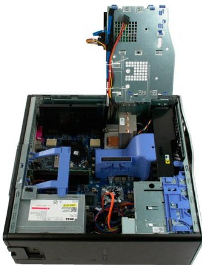
4. Lift the memory shroud straight up and remove the memory shroud from the computer.
