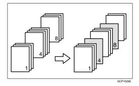
• Print on front side only Prints on the front side of slip sheets even if duplex printing is selected.
