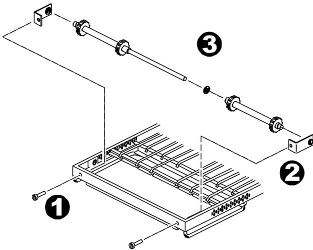
8. Reassemble the idler shaft into the conveyor. Make sure that the bronze washer is in place between the two sections of the shaft. See Figure 4-4.
