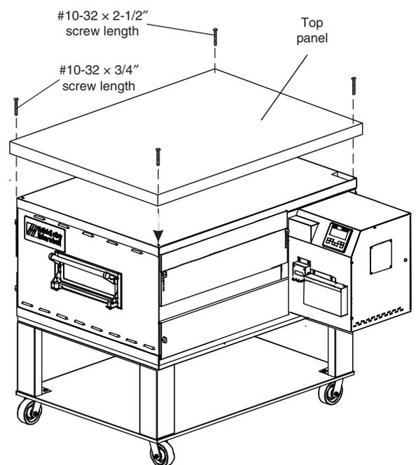
**NOTE:** DO NOT install top panel onto double or triple ovens until AFTER stacking the oven cavities. See Part B, Stacking.
