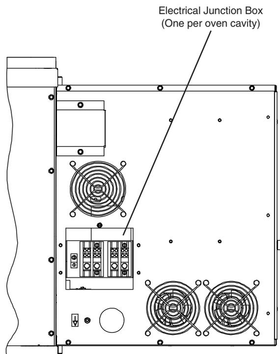
Figure 2-18. Utility Connection Locations for Electric Ovens
