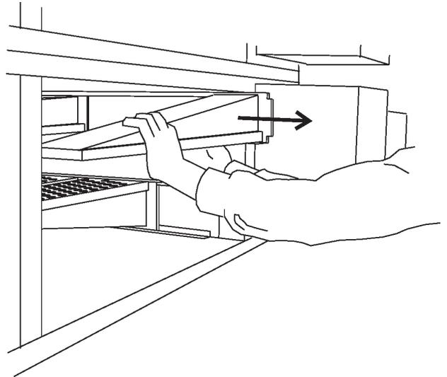
**Figure 4-3. Disassembling the Air Fingers**
