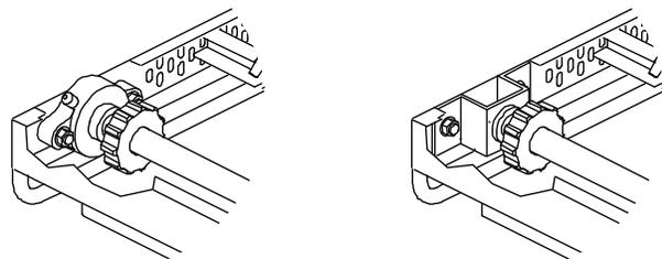
**Figure 4-6. Disassembling the drive shaft**
