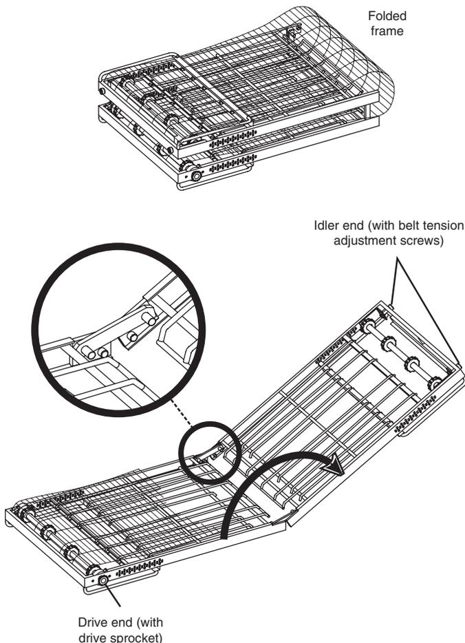
Figure 2-13. Conveyor placement
