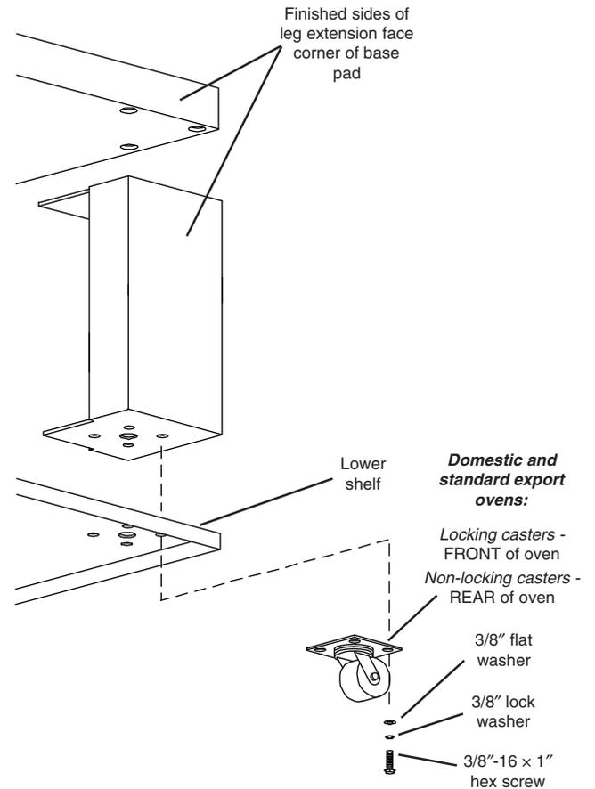
Figure 2-7. Base pad Installation
