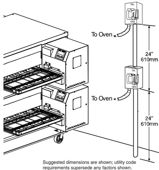
Figure 2-19. Typical PS840-Series Oven(s)
