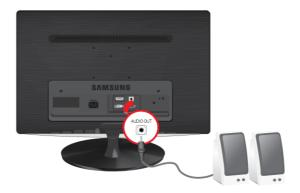
This product won't make any sound when only the HDMI cable is connected without a speaker connected.
