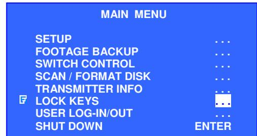
2. Select [LOCK KEY] option and press “Enter”
