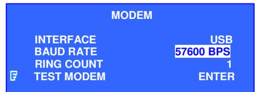
11.a.7. Press [OK] and back to modem sub-menu. Make sure the modem is connected and restart the modem if the modem is not ready.
