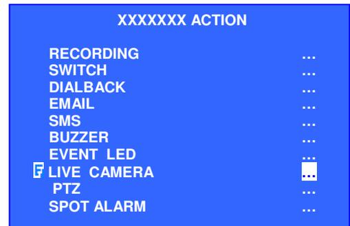
2. Select [ENABLED] option and use “Left” or “Right” button to enable (i.e. set the value to [YES]) live camera action.
