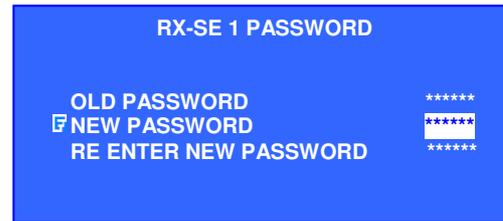
8. Input the new password and press **[END]**. Select **[RE ENTER NEW PASSWORD]** option and press “Enter”
