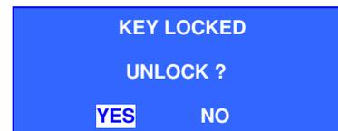
*\*NOTE: password is required if KEY LOCK PASSWORD is enabled.*
