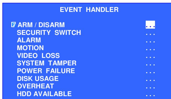
The event handler menu contain 9 functions (**ARM/DISARM**, **SECURITY SWITCH**, **ALARM**, **MOTION**, **VIDEO LOSS**, **SYSTEM TAMPER**, **POWER FAILURE**, **DISK USAGE**, **OVERHEAT** and **HDD Available**)
