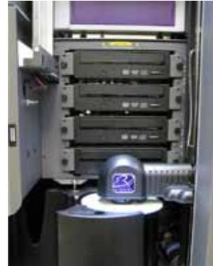
9. Manually, slightly rotate the **carousel** so that the distance between the edges of the carousel and the edge of the disc is equal on all four points, as shown.
