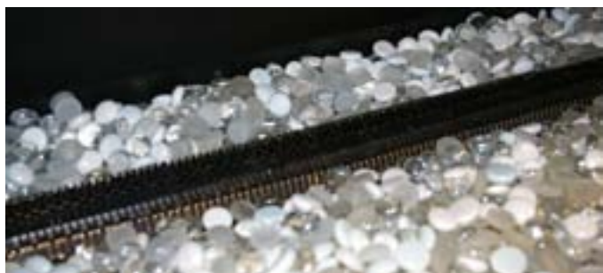
Figure 28. Installation of the Optional burner covers , (Place the covers end to end; do not overlap).
