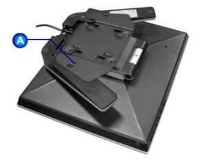
Fold the base and put the set-mount bracket into it. Align the set-mount interface holes with the holes in the base  $\bf A$  and secure it tightly with 2 screws.
