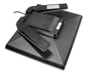
Fold the base and lay the area connected to cable face-down before putting the set-mount bracket into it. Align the set-mount interface holes with the holes in the base  ${\bf B}$  and secure it tightly with 4 screws.
