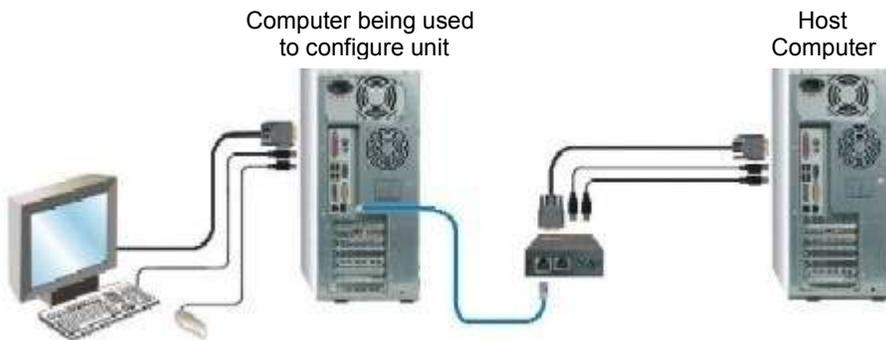
Figure 9. Connections for initial IP configuration
