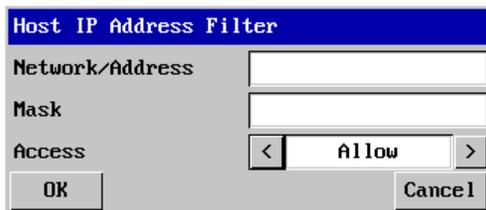
The image shows a dialog box titled "Host IP Address Filter". It has a blue title bar. Below the title bar, there are three input fields: "Network/Address", "Mask", and "Access". The "Access" field contains the word "Allow" and is flanked by left and right arrow buttons. At the bottom of the dialog, there are two buttons: "OK" on the left and "Cancel" on the right.
