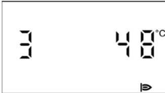
**Note:** If a boiler is not operational, the following appears in the display of the corresponding control unit:
