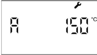
When a certain flue gas temperature is reached, e.g.: 302° F (150° C) (only with the Vitotronic 100, type GC1B).
