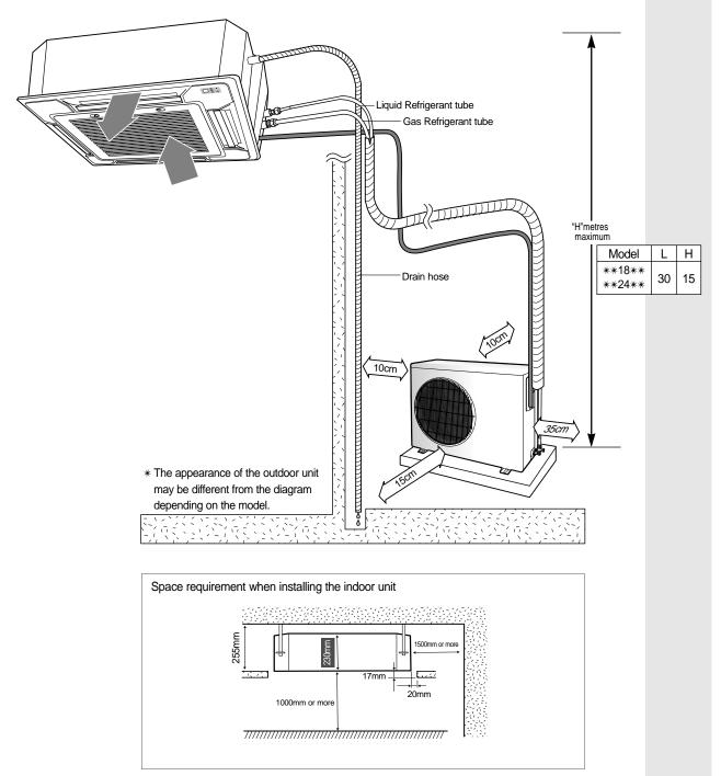
Respect the clearances and maximum lengths indicated in the diagram below when installing the unit.
