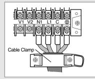
The indoor unit is powered from the outdoor unit via the connection cord.
