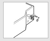
On delivery, the indoor unit is loaded with an inert nitrogen gas. All this gas must therefore be purged before connecting the assembly piping. To purge the inert gas, proceed as follows.
