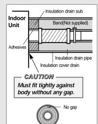
Care must be taken when installing the drain hose for the indoor unit to ensure that any condensate water is correctly drained outside.
