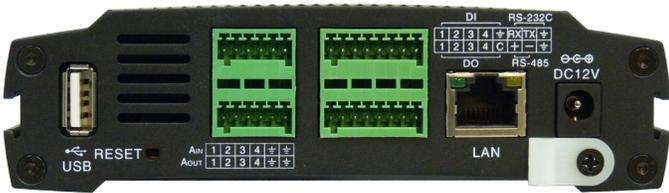
Connections to the encoder for audio in and out (microphone and speaker), D/I sensor, alarm, video out BNC, RS-232C, and RS-485 control are made through two 6-pin and two 8-pin terminal blocks. Vin1 is associated with Ain1 (microphone), Aout1 (speaker), D11 (sensor), DO1 (alarm output), and the first IP channel. Similarly, Vin2 is associated with Ain2, Aout2, etc. Attach peripheral devices to the terminal blocks as shown below. For detailed interface specifications, refer to the user manual.
