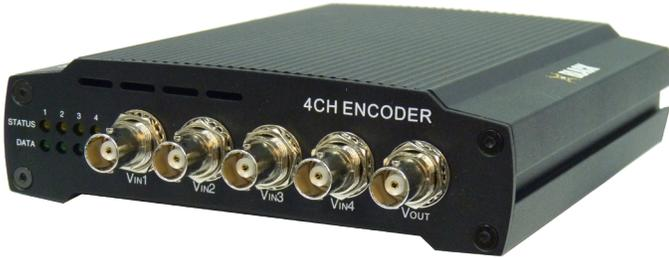
Connect video feeds from four analog cameras to the four Vin BNC connector (Vin1, Vin2, Vin3, Vin4) on the front of the encoder.
