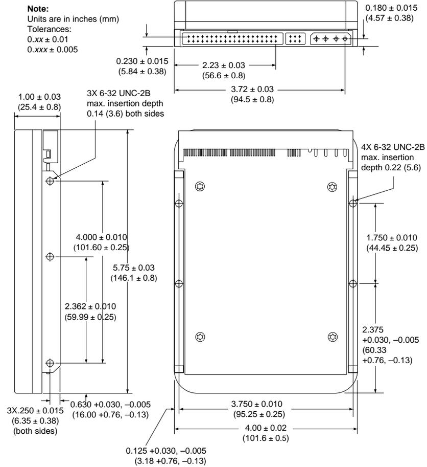
Figure 4. Mounting dimensions—top, side and end view
