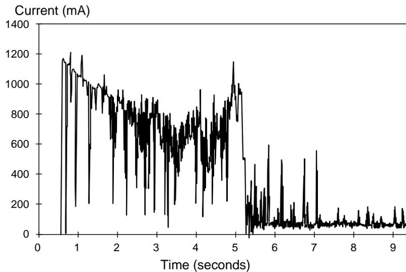
**Figure 2. Typical startup and operation current profile for the ST32122A, ST31722A and ST31012A**
