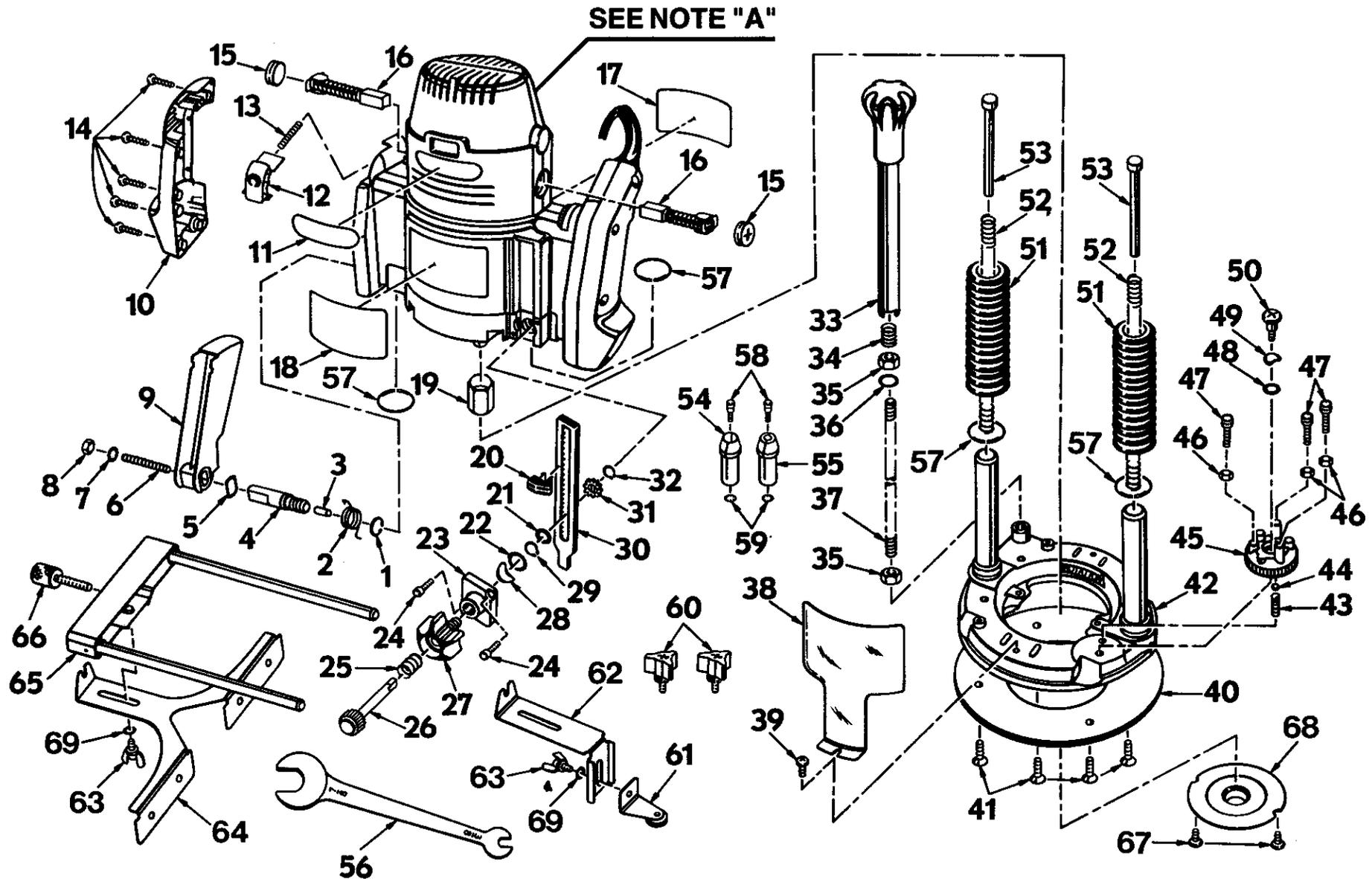
**NOTE: "A"** - The assembly shown represents an important part of the Double Insulated System. To avoid the possibility of alteration or damage to the system, service should be performed by your nearest Sears Repair Center. Contact your nearest Sears Retail Store for Service Center information.
