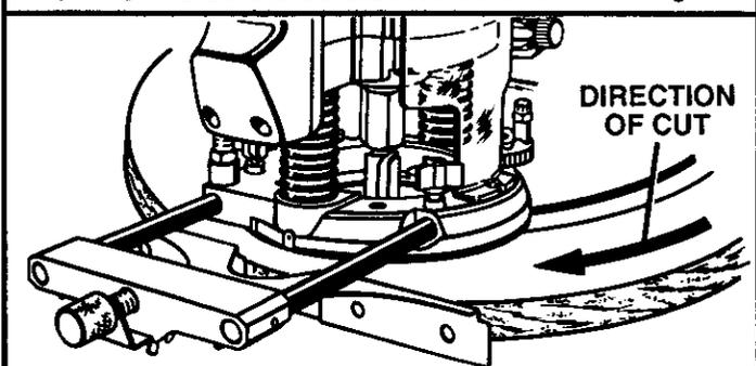
ROUTING INSIDE OF A CIRCLE WITH OPTIONAL EDGE GUIDE ATTACHMENT Fig. 25
