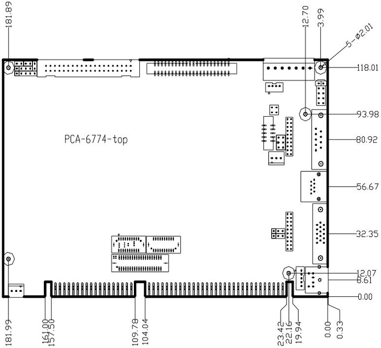
*Figure 1.1: Board layout: dimensions (component side)*
