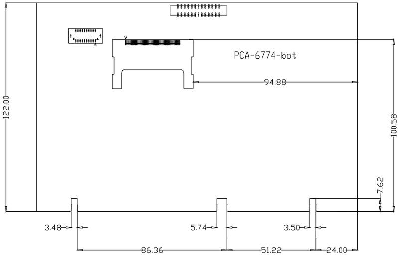
**Figure 1.2: Board layout: dimensions (solder side)**
