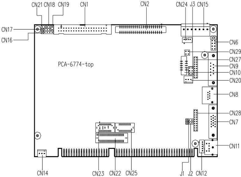
**Figure 2.1: Jumper & Connector locations**
