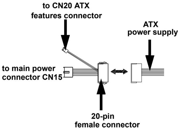
*Figure 2.3: Wiring for ATX soft power switch function*
