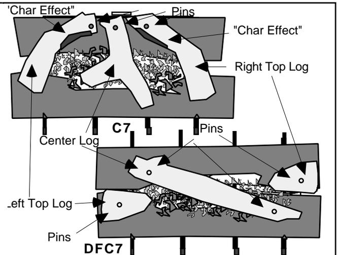
**Volcanic Ash Placement:** Place **VOLCANIC ASH** only on the firebox floor. **NEVER PLACE VOLCANIC ASH** (or any material other than the **EMBER MATERIAL** provided) **ON TOP OF BURNER!**
