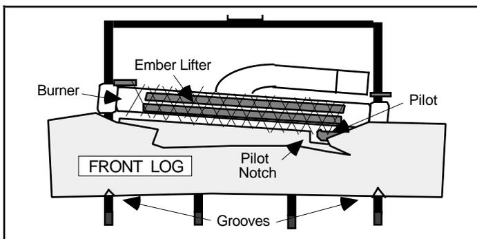
1. **FRONT LOG:** Align LOG GROOVES with Grate Teeth. Slide leading edge of FRONT LOG beneath EMBER LIFTER maintaining PILOT NOTCH to PILOT position as shown.
