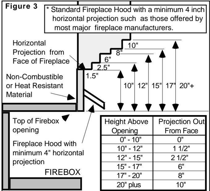
**IF YOU CANNOT MEET THESE MINIMUM CLEARANCES YOU MUST OPERATE HEATER WITH CHIMNEY FLUE DAMPER OPEN (Operate as a VENTED Heater - See Page 3).**
