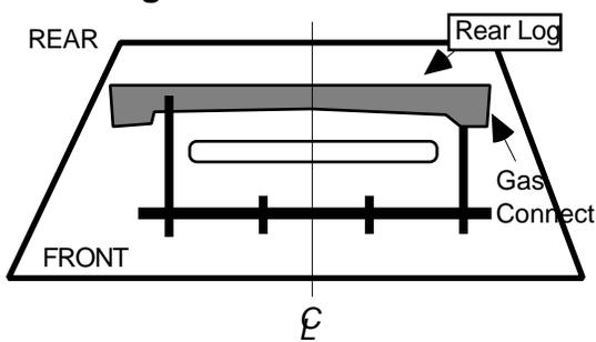
With Rear Log on grate, place grate/control assembly inside firebox or approved enclosure. Center left to right with the back portion of the grate assembly as far to the rear of the firebox as possible.
