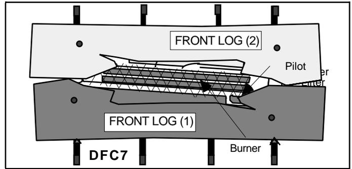
**EMBER MATERIAL:** With the **FRONT** and **REAR LOGS** on the Grate as shown, pull apart the **EMBER MATERIAL** into **long loose, thin pieces** and drape them over the **EMBER LIFTER**. The pieces **should be no more than one to two pieces of ember material in depth**. To enhance ember performance, after approximately 5 minutes of burn time, gently loosen and lift **EMBER MATERIAL**.
