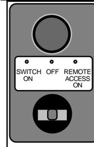
Manual: Switch from OFF to SWITCH ON; SWITCH ON to OFF
