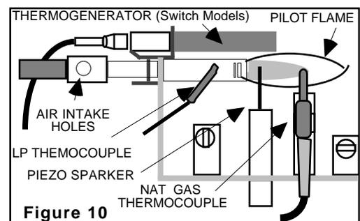
**IMPORTANT SERVICE TIP!** Obstructed Pilot Air Intake Ports result in an improper gas/air mixture and a weak pilot flame. **Weak pilot flame is the NUMBER 1 SERVICE ISSUE RE NUISANCE SHUT-OFF.** Using canned compressed air, pipe cleaner or an artist's brush, clean out the opposing Air Intake Ports located at base of Pilot (where gas supply line attaches to pilot). (Figure 10)
