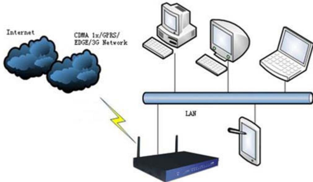
Diagram 2.3-2: Schematic diagram for application in SOHO
