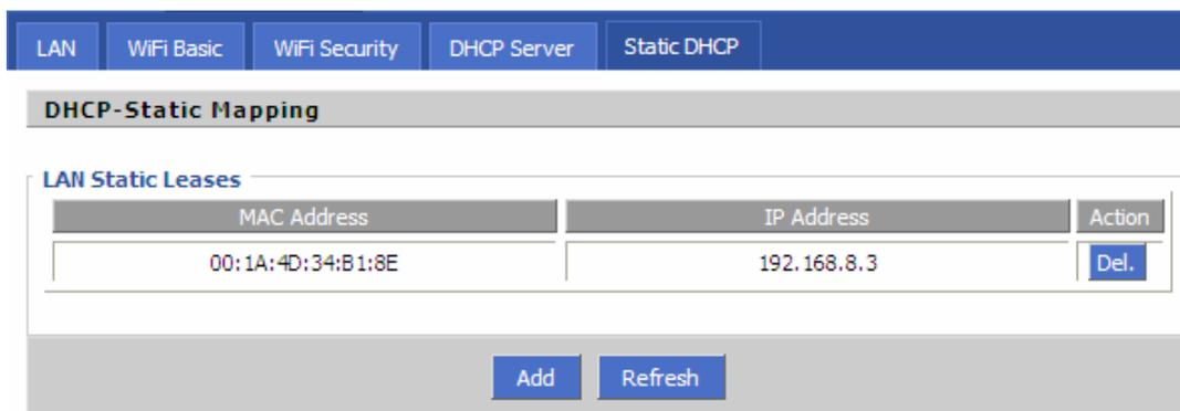
Fig. 3.3.3.3-1: DHCP Configuration Interface
