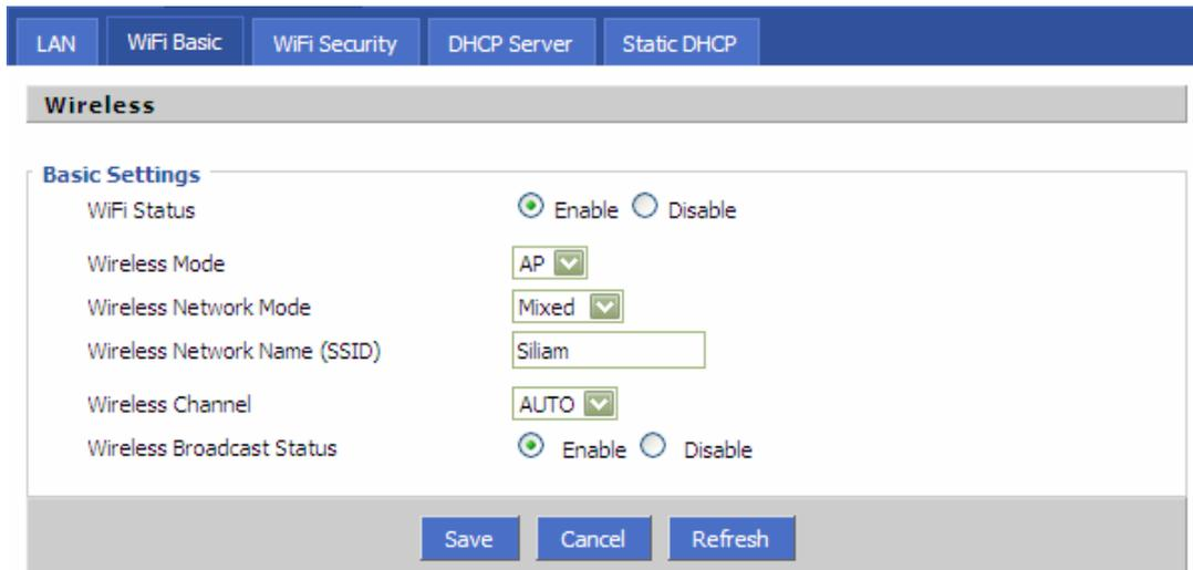
Fig. 3.3.3.2: Wireless configuration interface
