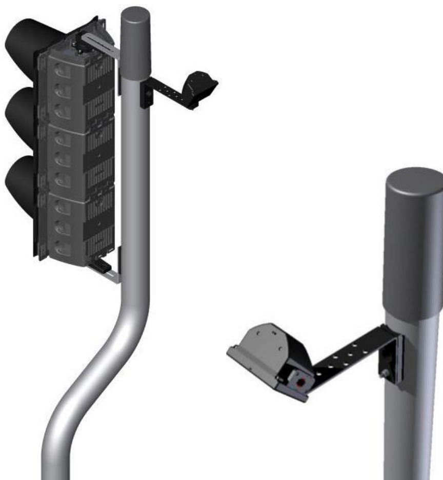
Figure 29 : Cranked Pole Kerbside Installation and Bracket Detail
