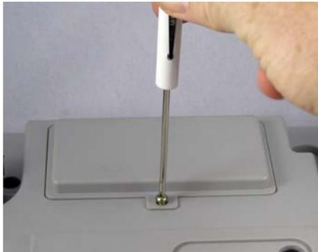
Remove the screw holding the battery compartment lid on the bottom of the scale.
