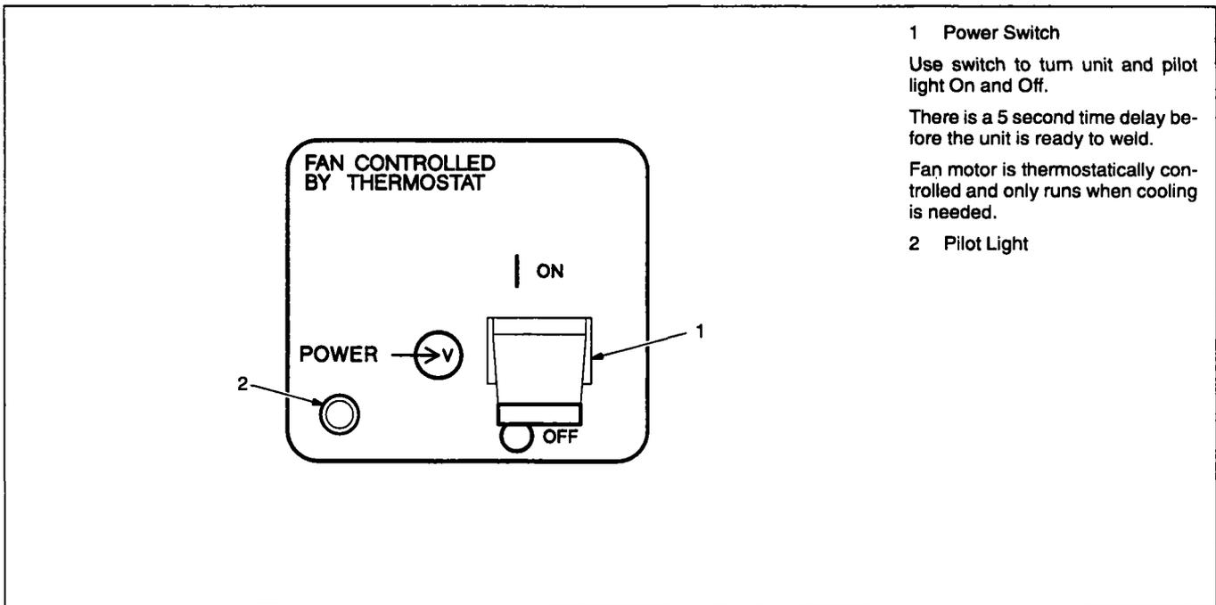
Figure 4-11. Power Switch And Pilot Light
