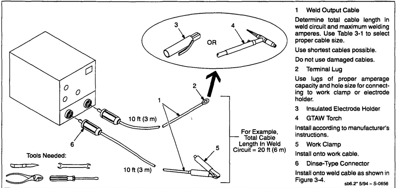
Figure 3-3. Selecting And Preparing Weld Output Cables
