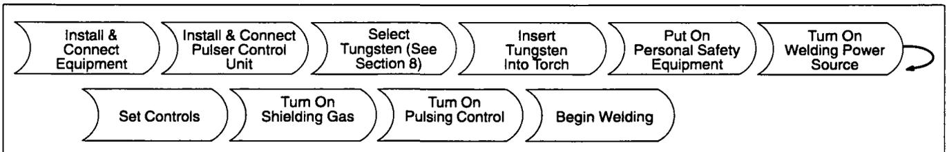
**Figure 4-14. Sequence Of Gas Tungsten Arc Welding – Pulsed (GTAW-P)**
