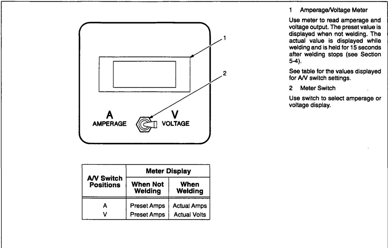
Figure 4-10. Amperage/Voltage Meter And Switch (Optional)
