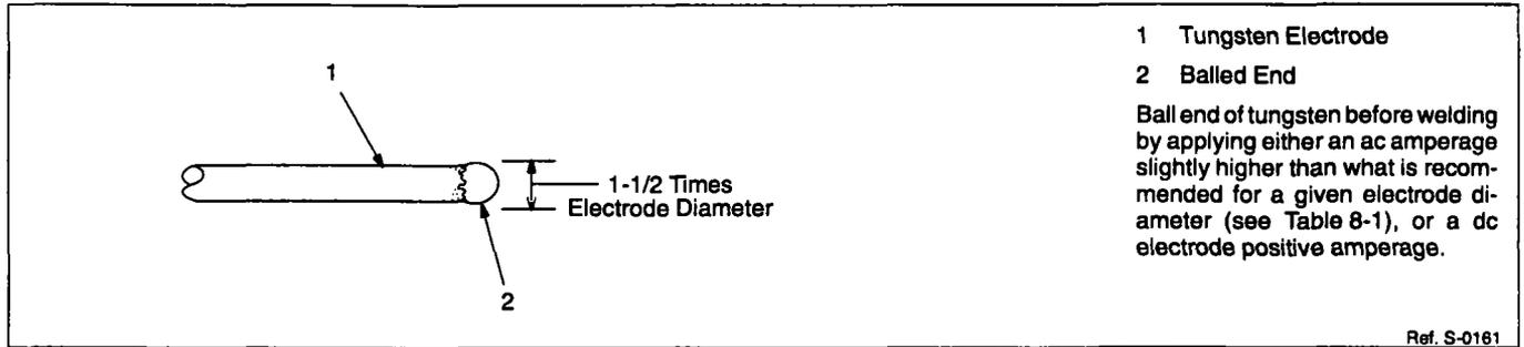
Figure 8-1. Preparing Tungsten For AC Or DC Electrode Positive (DCEP) Welding
