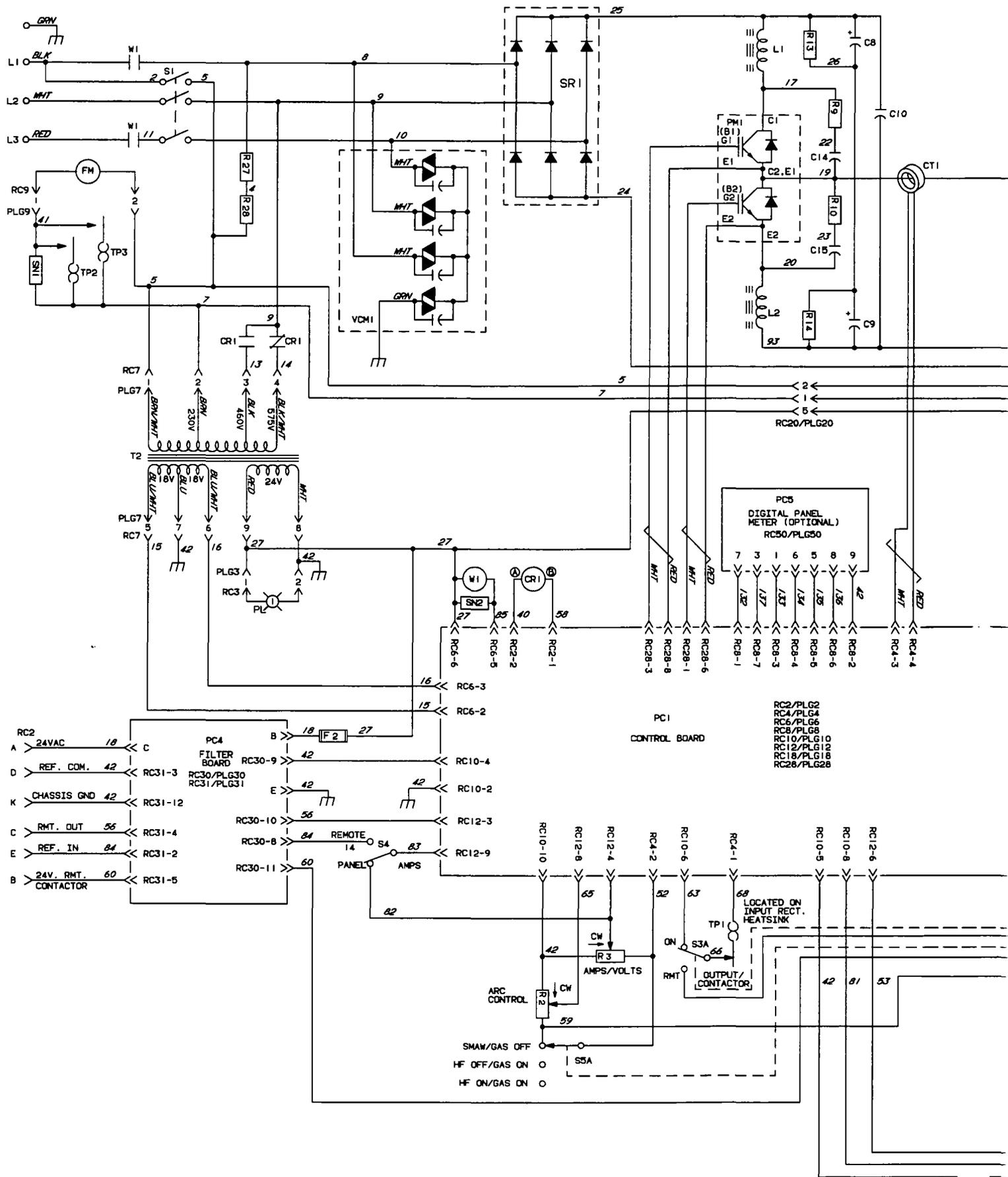
Figure 6-2. Circuit Diagram For 460/575 Volt Models
