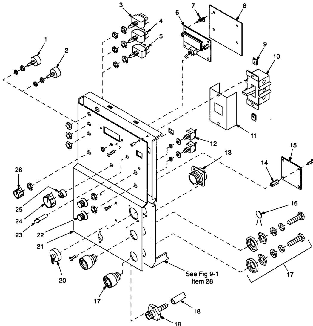
**Figure 9-3. Panel, Front w/Components**
