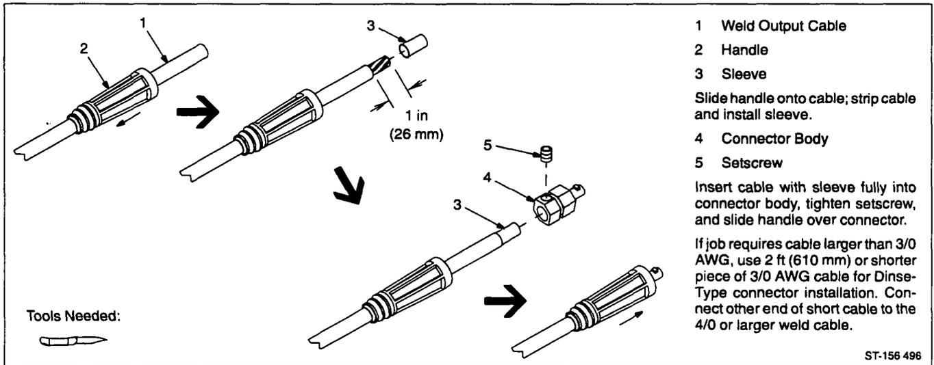
Figure 3-4. Dinse-Type Connector Assembly
