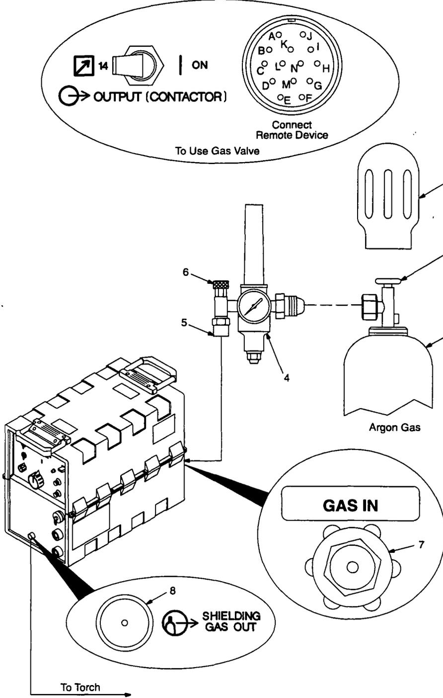
Obtain gas cylinder and chain to running gear, wall, or other stationary support so cylinder cannot fall and break off valve.
