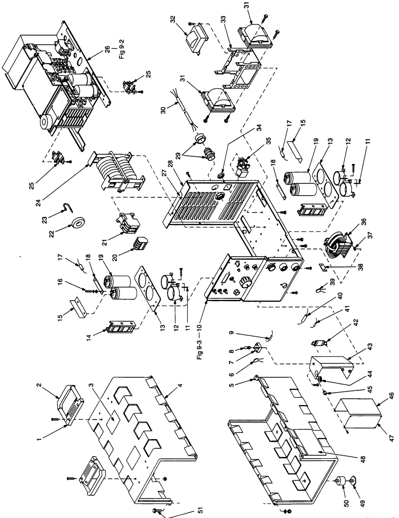
Figure 9-1. Main Assembly (208-230/460V Model Illustrated)
