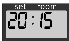
E: When the 4-digit stops blinking, the setting has been locked to the indicated value.
