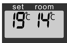
F: The required temperature on the left, the measured temperature on the right.
