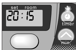
G: The TIMER indicator light indicates that the timer function has been switched on.
