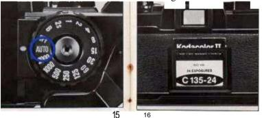
Turn the shutter speed dial to the "AUTO" position (Fig. 15). A convenient memo holder is provided on the back of your camera. Whenever you load new film, just cut off the top of the film box and put it in the memo holder as a reminder. (Fig. 1 6).
