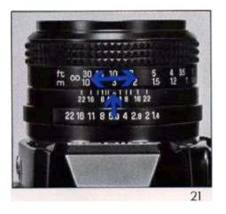
You can also focus indirectly. Actually measure or estimate the distance to the subject and set the lens focus ring to the appropriate setting (Fig. 21).
