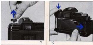
Pull out the film rewind knob until the camera back pops open (Fig. 9). Then drop a film cartridge into the film chamber with its protruding end facing the bottom of the camera (Fig. 10). Push in the film rewind knob and slightly turn the knob in either direction until it catches the film cartridge spool. Insert the trimmed end of the film into a slot of the multi-slotted take-up spool\_\_\_\_\_
