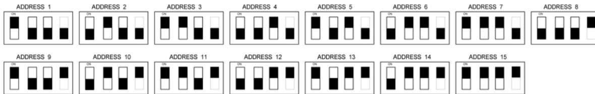
The black portion of the DIP identifies the switch actuator. An address of 7 is set when actuators of the DIP switch are “up” on positions 1, 2 and 3.
