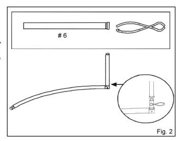
3. Connect two top rail sections together. Repeat for the other top rail sections as shown in Fig 3.
