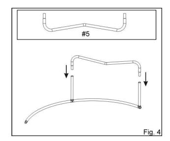
5. Turn over the 4 sub-assembled sections and connect them together. Note that at this stage the sections can still become easily separated. The assembly will become rigid only when the trampoline mat is assembled to the frame.
