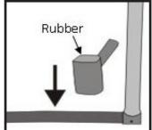
2. Do **NOT** disassemble the T-section (#4) and the top rail (#3); you can keep it as it is. It is not necessary and it will make re-assembly easier.
