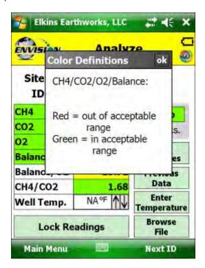
These ranges are programmable for each well by utilizing the Configuration Editor as detailed in section 7.
