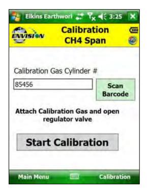
5) Attach the calibration gas to the Static sample port located on the front of the Envision® gas analyzer and open the regulator valve. Elkins Earthworks® strongly recommends the use of a Demand Flow regulator. Warning — attach the calibration gas only to the Static port. Do not attach the calibration gas to the Exhaust, Impact or Available ports. Pressures above 200" H20 on any port other than the static pressure port may result in a damaged pressure sensor.
