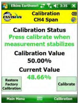
a. If the "Current Value" is between 0% and 20% (relative) of the calibration gas value then the Trimble handheld computer will adjust and store your calibration once the user taps the "calibrate" button.
