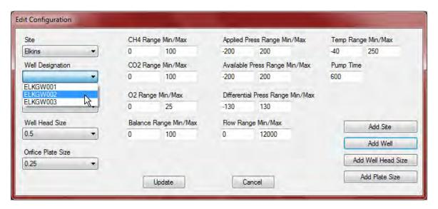
The user may now select the wellhead type, wellhead size, and orifice plate size. If the user desires to type in the flow in the field they may use the User defined type under "Well Designation". If the default list of "Well Head Sizes" or "Orifice Plate Sizes" does not include the desired size then the user may add a new size using the "Add Well Head Size" and "Add Plate Size" buttons.
