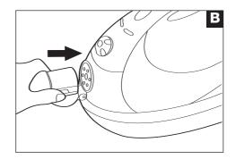
Please refer to the accessory assembly section for full descriptions on how to attach tubes and nozzles.
