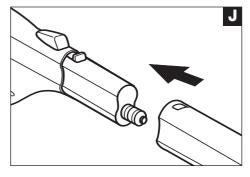
2 To connect the desired accessory directly to the hose handle, slide the handle into the accessory head or tube until it locks in place .
